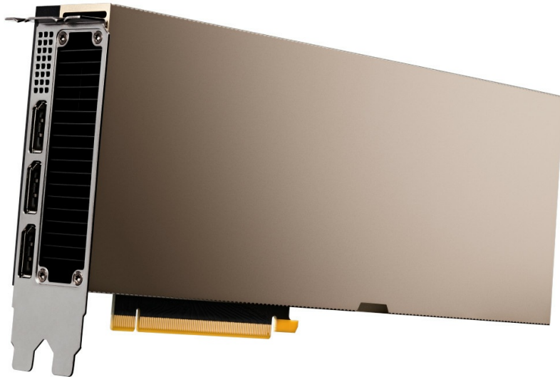
Figure 9. ThinkSystem NVIDIA A40 48GB PCIe Gen4 Passive GPU
