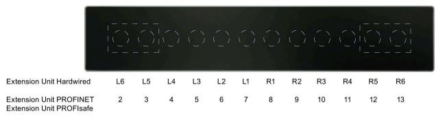
With Extension Unit PROFINET and Extension Unit PROFIsafe, the slots are numbered similar to the display in TIA Portal in ascending order from left to right. The numbering in this figure corresponds to STEP 7 (TIA Portal) as of V15; for V14, the numbering of the slots from 1 to 12 applies.
