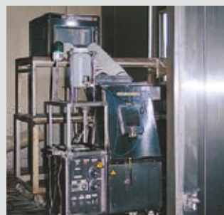
Dust and vapour test*4 Operating in dust and vapour at a temperature of 40°C and a relative humidity of 95 %
