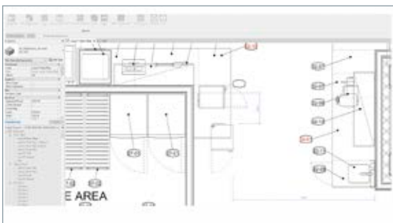
Check that the open doors of the microwaves do not interfere with the pathways
