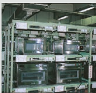
Endurance test at intermittent operation*4 On (60s) and off (30s) 200.000 times; On (20s) and off (10s) 200.000 times
