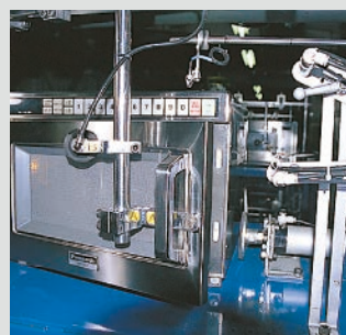
Endurance test of door (opening and closing)*4 400.000x opening and closing the door
