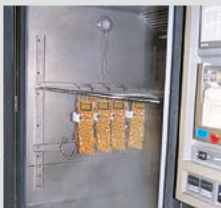
Circuit boards stress test*4 Temperature of -40°C to +85°C, relative humidity 85 %
