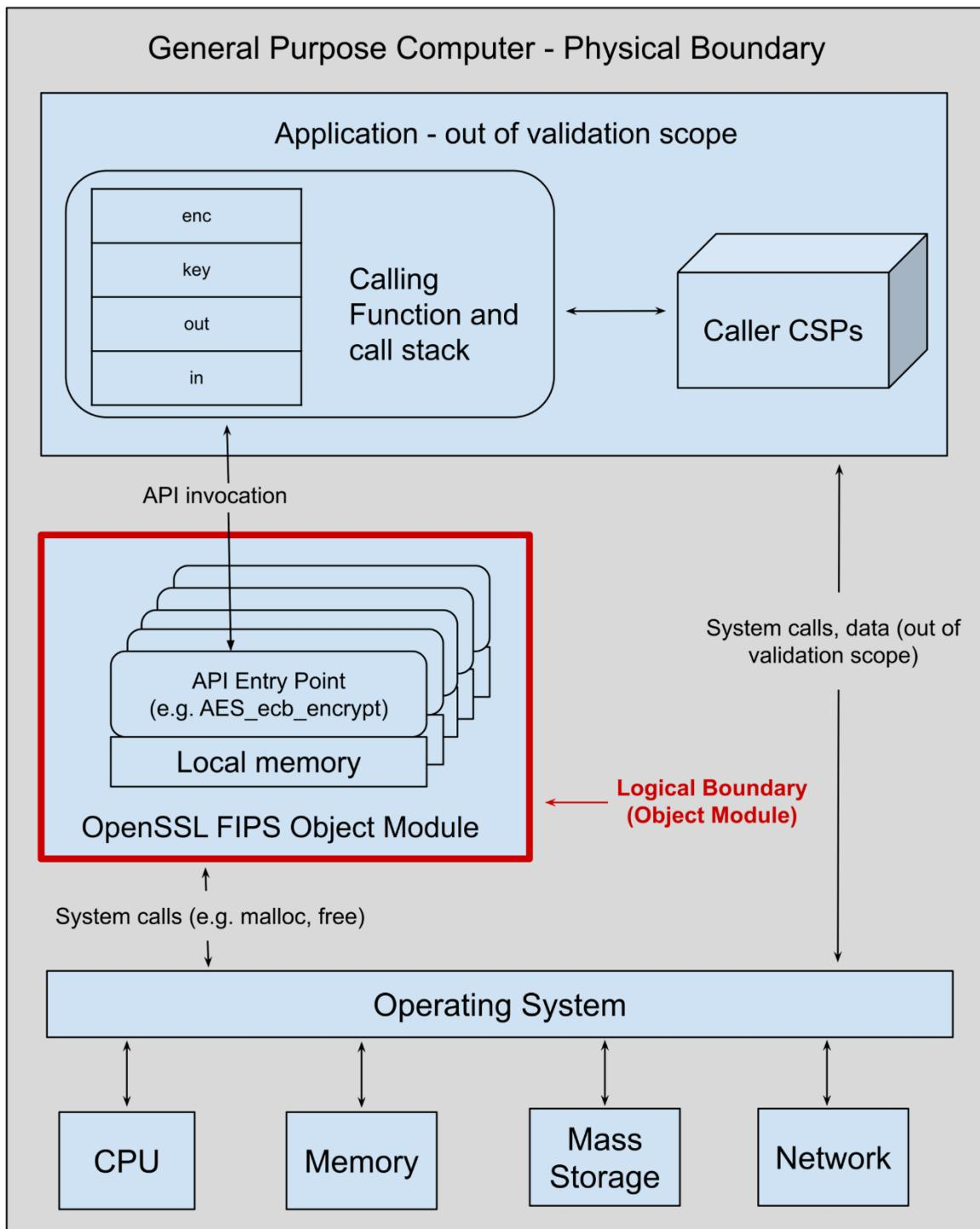
Figure 1 - Module Block Diagram
