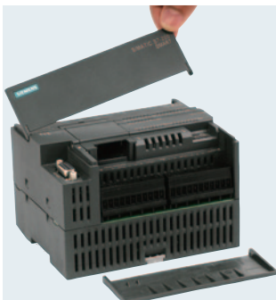
Remove the cover board of terminal
