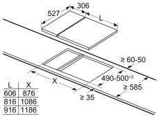
When installing a Domino unit right next to a hob, an assembly kit (HEZ394301) is required.
