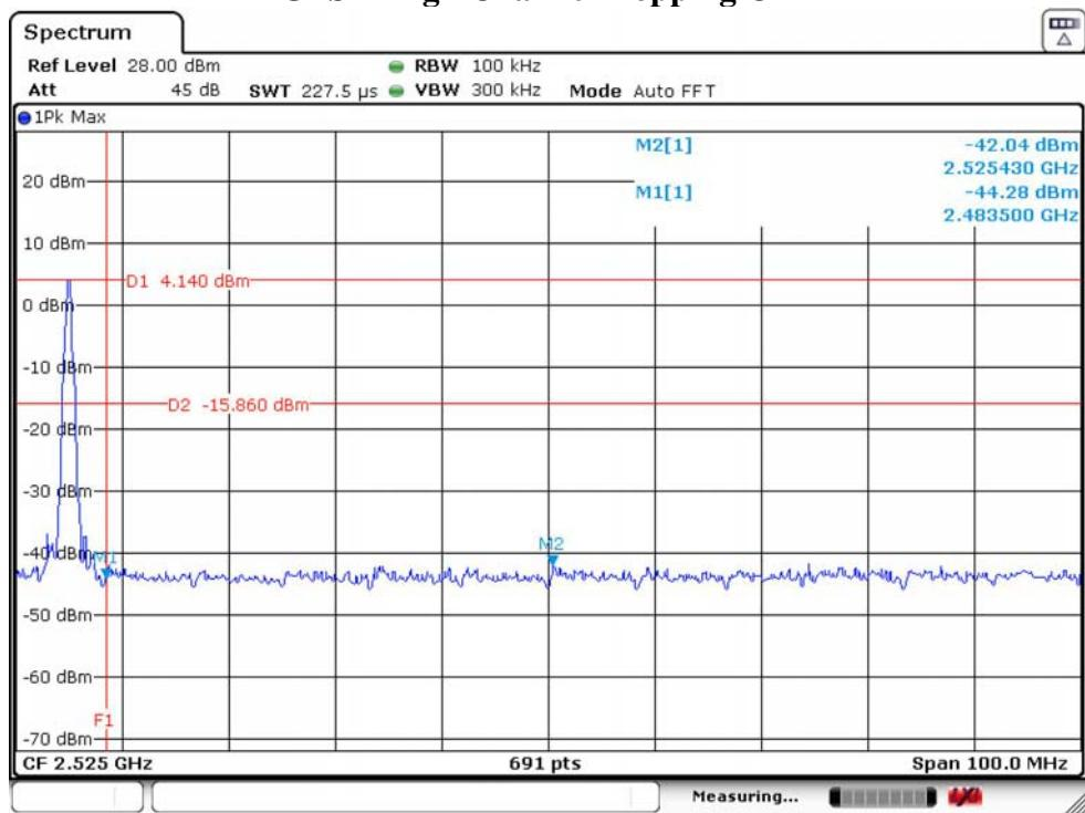
**GFSK Low Channel Hopping ON**
