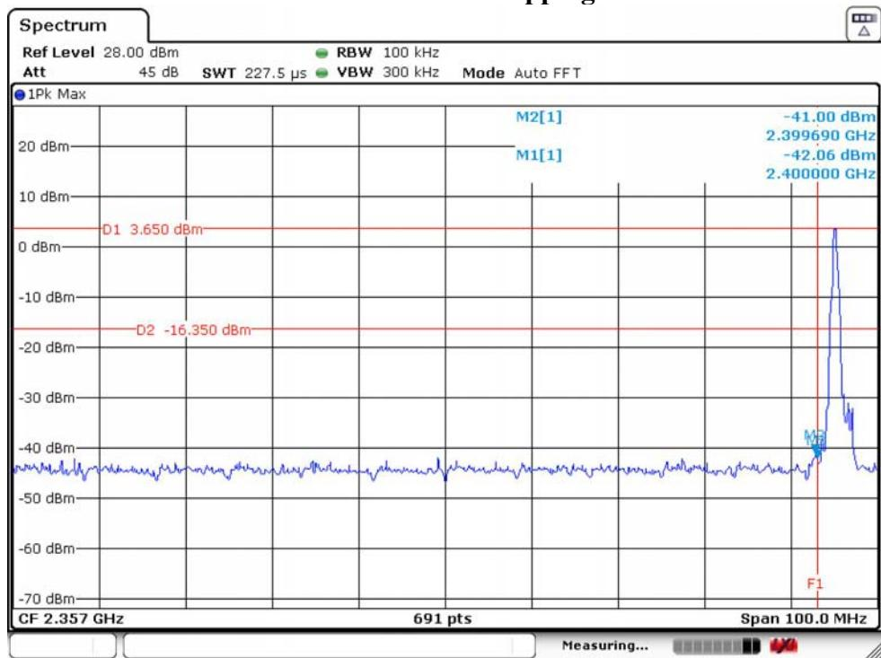
**GFSK High Channel Hopping OFF**
