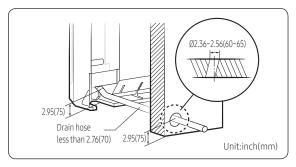
6 Refrigerant and drain pipes and cables should go through the hole located at the on the back of the unit at the bottom.
