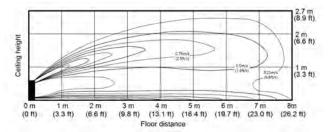
• Heating Air Velocity distribution (Discharge angle: 4 degree)
