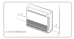
When you install the indoor with side-pipe connection, please make space more than 11.81 inch (300mm) from the wall.
