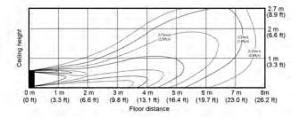
• Cooling temperature distribution (Discharge angle : 40 degree)
