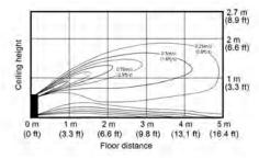
Heating Air Velocity distribution (Discharge angle: 4 degree)
