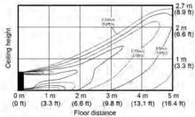
• Cooling temperature distribution (Discharge angle: 40 degree)
