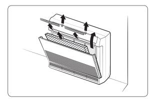
4 The body front should be opened to connect pipes.
