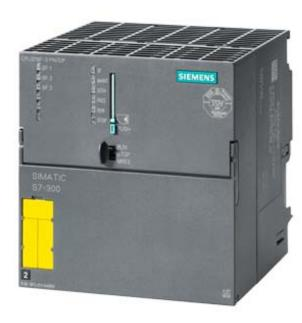
SIMATIC S7-300 CPU319F-3 PN/DP, Central processing unit with 2.5 MB work memory, 1st interface MPI/DP 12 Mbit/s, 2nd interface DP master/slave 3rd interface Ethernet PROFINET, Micro Memory Card required
