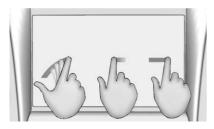
Fling or swipe is used to scroll through a list, pan the map, or change page views. Do this by placing a finger on the display then moving it rapidly up and down or right and left.
