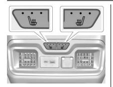
If available, the buttons are on the rear of the center console. To operate, the vehicle must be on.
