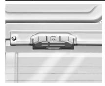
Once the glass stow retainer handle is in the locked position, the rear glass is securely stored.
