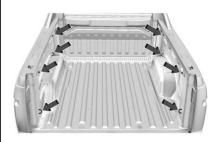
This vehicle is equipped with eight fixed cargo tie-downs.
