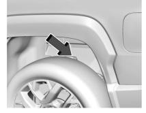
1. Reach around the tire to find the emergency manual charge cord release.
