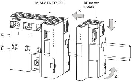
Figure 6-1 Installing the DP master module
