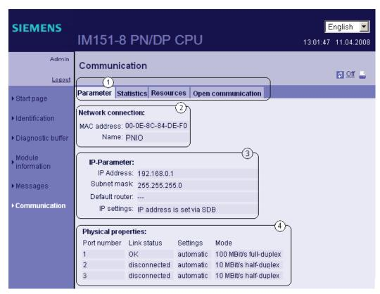
Figure 3-12 Parameters of the integrated PROFINET interface
