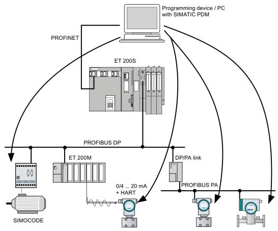
Figure 3-1 IM 151-8 PN/DP CPU data set routing
