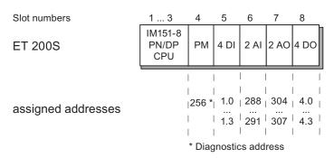
Figure 7-3 Example of address assignment for I/O modules
