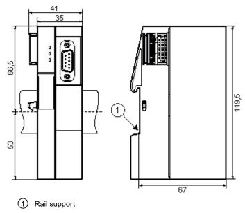
Figure A-2 DP master module dimensional diagram
