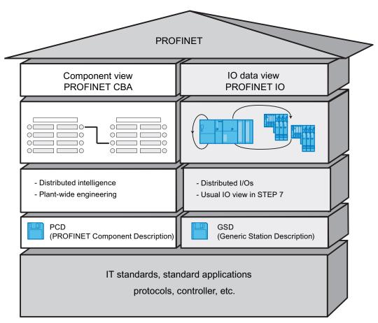
Figure 4-1 Extent of PROFINET IO and Component-Based Automation
