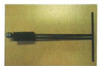
Figure 1 – MVG COMOSAR Validation Dipole
