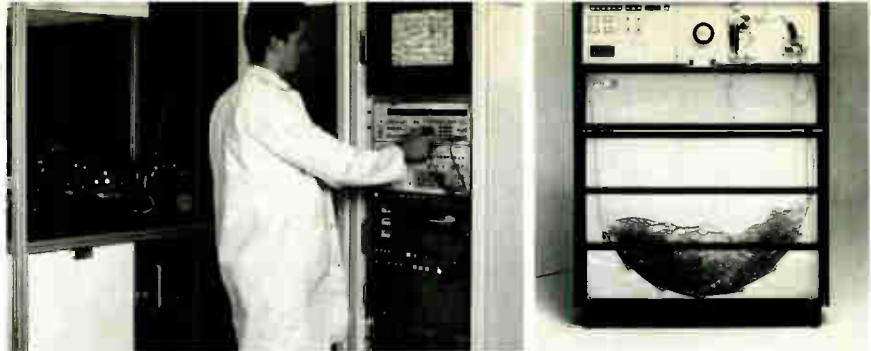
Left: OD&ME's compact disc master recorder MR 100; right: Lyrec loop-bin master P-4400. See page 153
