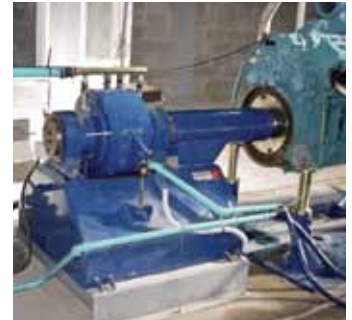
Typical dynamometer applications, testing diesel engines
