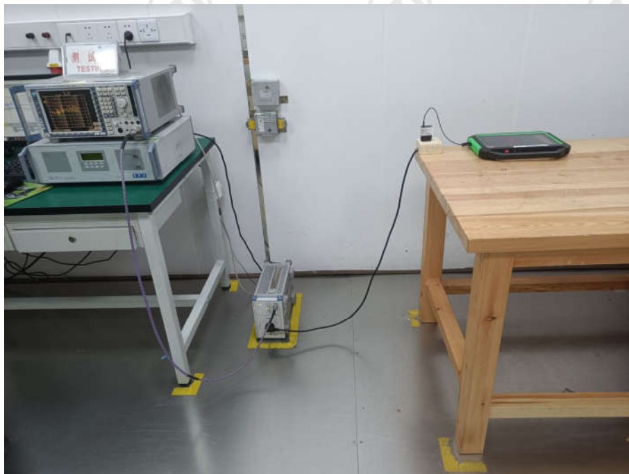
Conducted Emissions Test Setup
