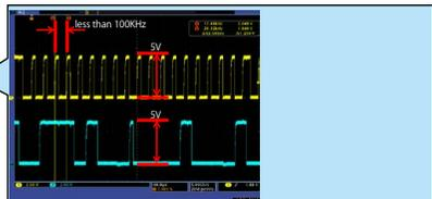
This diagram shows an example of the DDC communication waveform.
