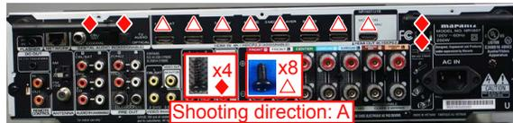
(2) Remove the connector PCB.
