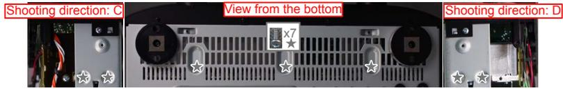
(2) Cut the wire clamps, then remove the CORD HOLDERS and connectors. Remove the screws. Remove the FFC.
