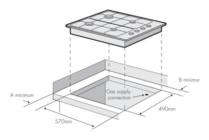
Walls around cooktop must be heat resistant for temperatures up to 90°C to a height of 150mm above the bench top.
