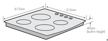
Note: Connection type - hardwired Maximum power load 6.0kW
