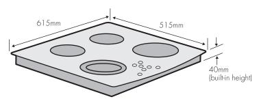
Note: Connection type - hardwired Maximum power load 5.9kW
