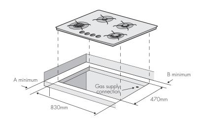
Walls around cooktop must be heat resistant for temperatures up to 90°C to a height of 150mm above the bench top.
