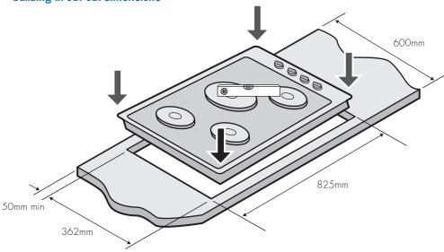
**Note:** Any walls surrounding the cooktop are to be heat resistant up to  $90^{\circ}\text{C}$ , up to 150mm high eg. ceramic tiles
