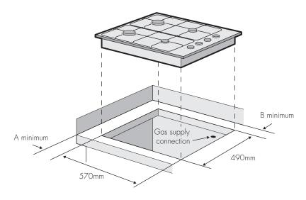
Walls around cooktop must be heat resistant for temperatures up to 90°C to a height of 150mm above the bench top.
