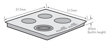
Note: Connection type - hardwired Maximum power load 6.5kW
