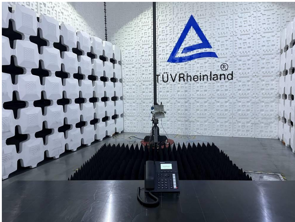
Photograph 2: Set-up photo for Radiated Emission, Above 1GHz
