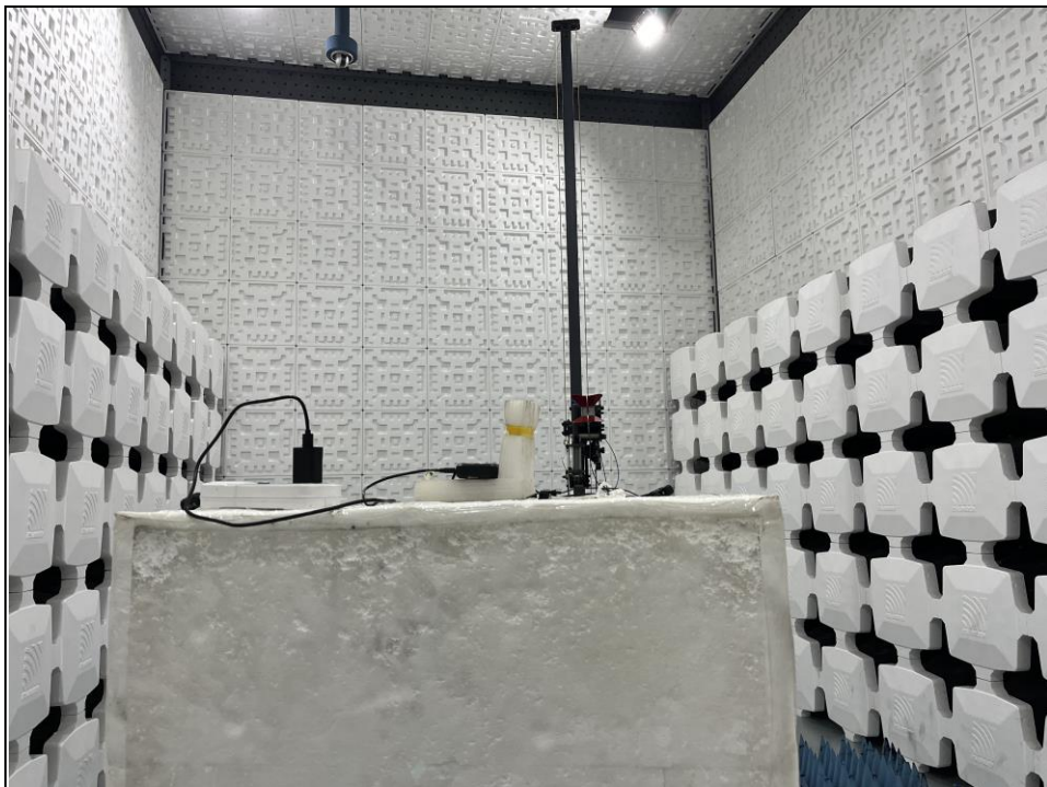
Radiated emission test: Frequency Range < Above 1GHz >
