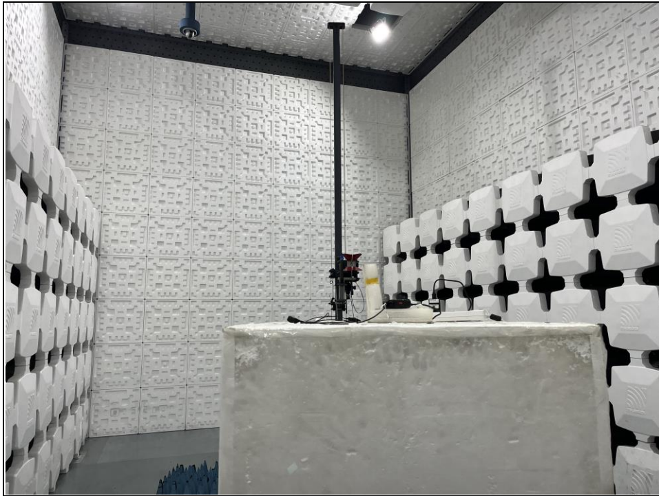
Radiated emission test: Frequency Range < 9KHz- 30MHz >
