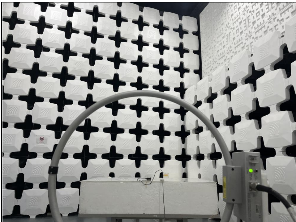
Radiated emission test: Frequency Range < 9KHz- 30MHz >
