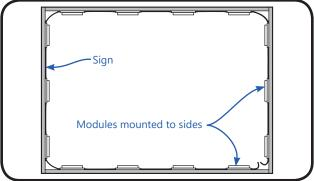
(1) Determine location of where LED modules will be mounted based on sign dimensions (see chart). If mounting on bottom of sign, the use of a riser will be needed (minimum 1/8 in. distance between bottom surface and module).
