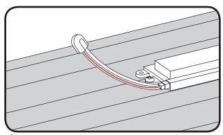
2 Cap all exposed wires with appropriate end caps or apply electric grade (non-corrosive) silicone for additional weather protection.
