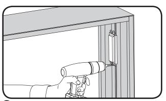
Use rivets, screws, or silicone to secure each module within the sign. Use #6 (M3) or #8 (M4) screws, 1/8-inch (3.2 mm) rivets, or silicone.
