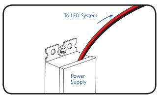
1) Run a wire from the Power Supply and connect to the first LED module on the strip.
