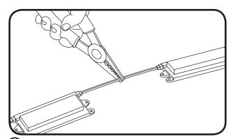
(2) Determine how many modules are required for your application and cut where necessary.
