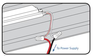
2 Connect the red stripe wire (+) of the LED system to the red wire (+) of the power supply. Connect the white wire (-) of the LED system to the black or blue wire (-) of the power supply.
