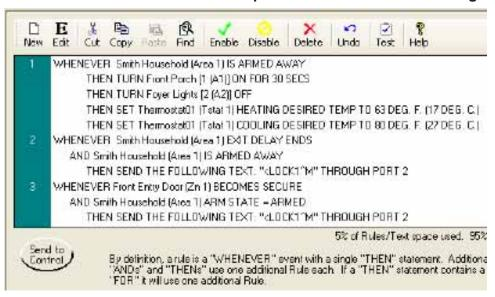
Rule 1 - When the System is Armed to Away mode this rule will turn on the Flood lights for 30 sec., turn off the Foyer Lights, and change the HVAC Thermostat Settings. This is typical of an Energy Save type of rule.
