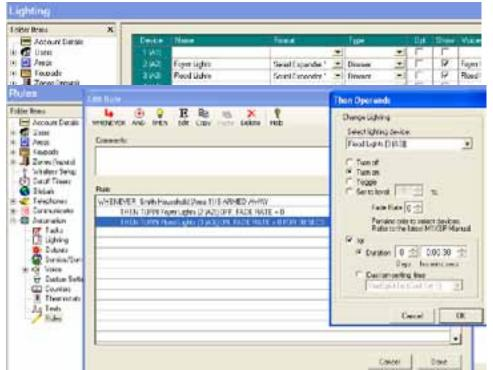
The Rule shown controls 2 lights when the System is Armed Away.
