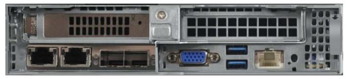
The H610S is a 1U storage node with 12 NVMe drives of sizes 960GB, 1.92TB, or 3.84TB with the option of drive encryption. A minimum of four H610S nodes are required to form a cluster. It delivers around 100,000 IOPS per node with a 4K block size. The following figure depicts a front and back view of an H610S storage node.
