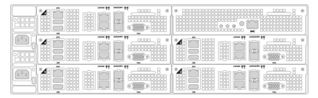
Each node has its own network, IPMI, USB, and VGA ports.
