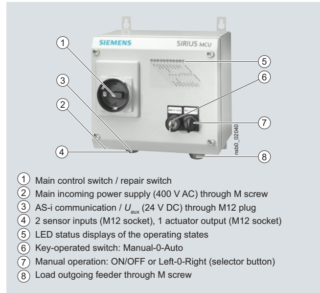
MCU for AS-i, metal enclosure, electromechanical switching
