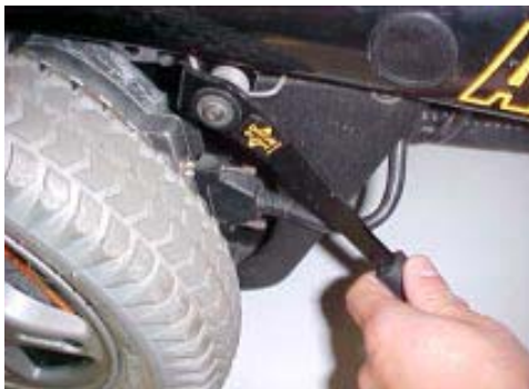
Figure 2. Engage and Disengage Brake lever, while your meter leads are connected to pins 9 and 10. You should hear an audible come on, then off while performing this test.
