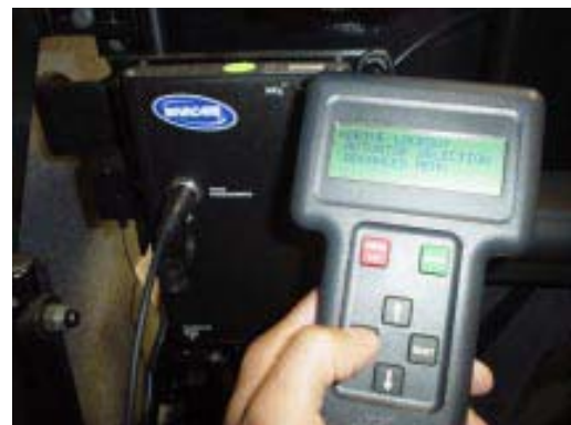
Remote programmer 5-pin connector can be used with the MK5 TAC and TRCM.
