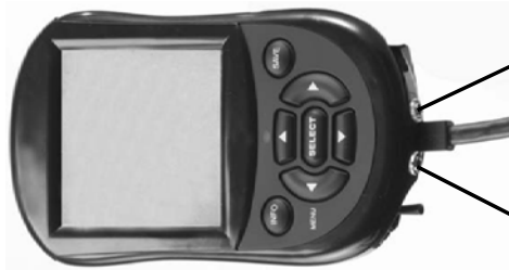
Remote On/Off Switch Port Mode/Actuator/ Drive Select Switch Port
