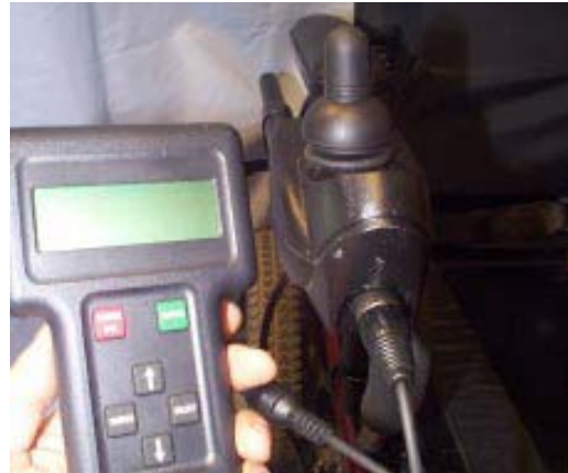
Remote Programmer 3-pin connector used for RII, RII-LP, and all MK5 & MK6 Electronics.
