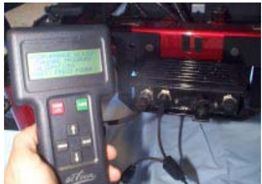
Remote Programmer 5-pin connector used for all MKIV electronics, and MK5 accessories.
