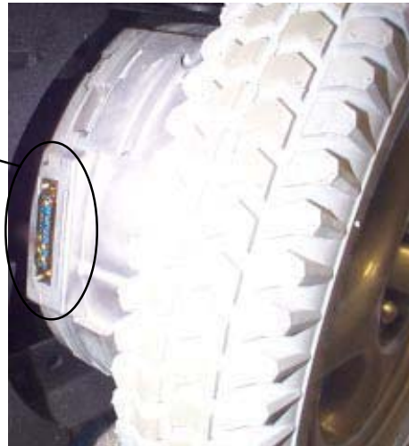
Figure 1. Motor Connector with numbered pins.
