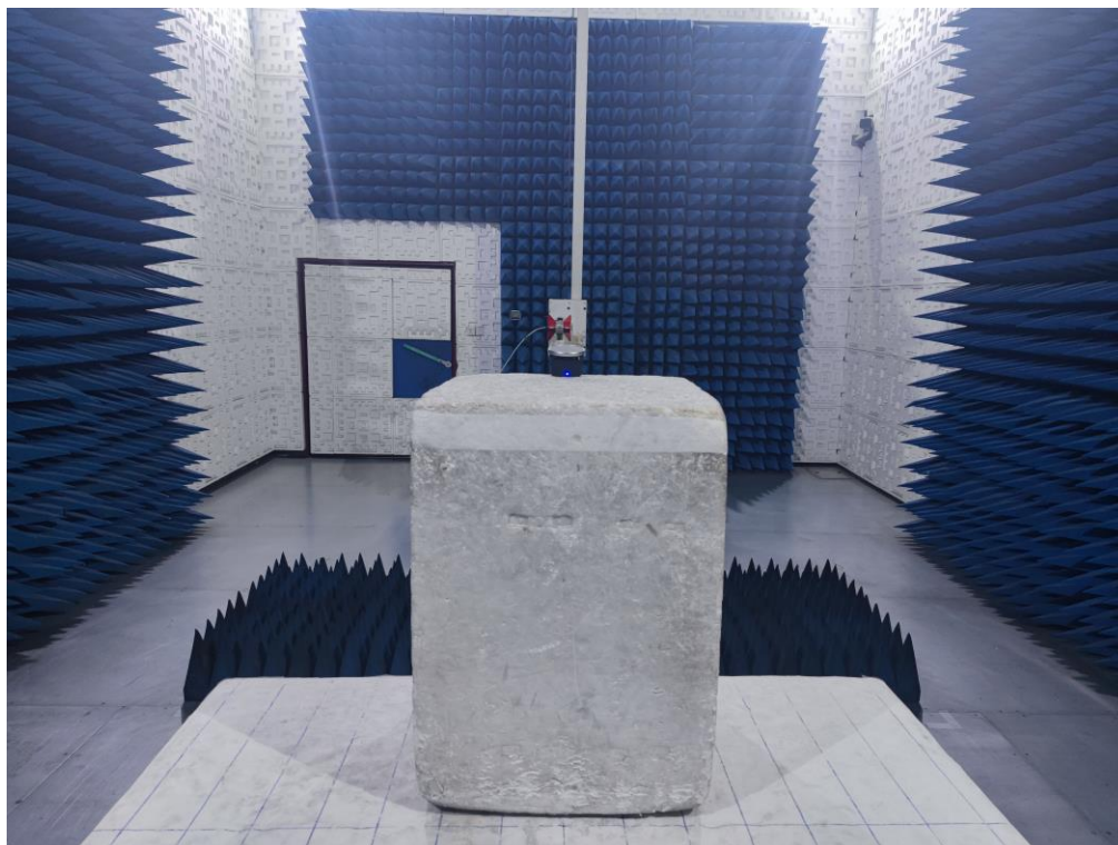
RADIATED EMISSION TEST SETUP ABOVE 1GHz
