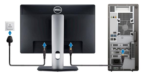
(i) **NOTE:** If you ordered the computer with a discrete graphics card, the HDMI and the display ports on the back panel of the computer are covered. Connect the display to the discrete graphics card.
