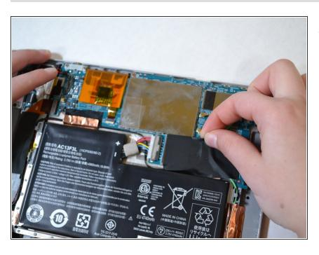
Remove the black tape connecting the battery to the motherboard.
