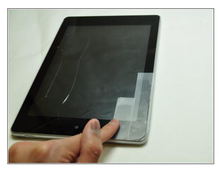
Add strips of tape to the sides of the device.
