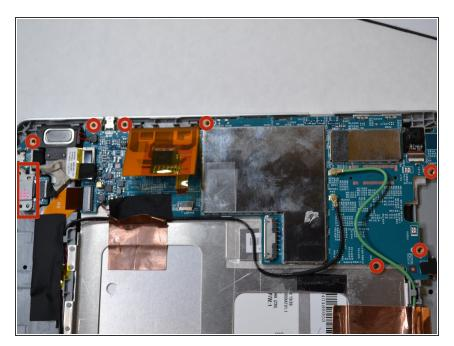
Use a Phillips #000 screwdriver to remove the screws around the perimeter of the motherboard.
