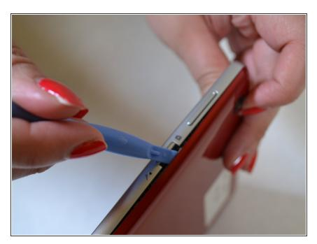
Remove the back cover by lifting with a plastic opening tool, below the camera button slot.
