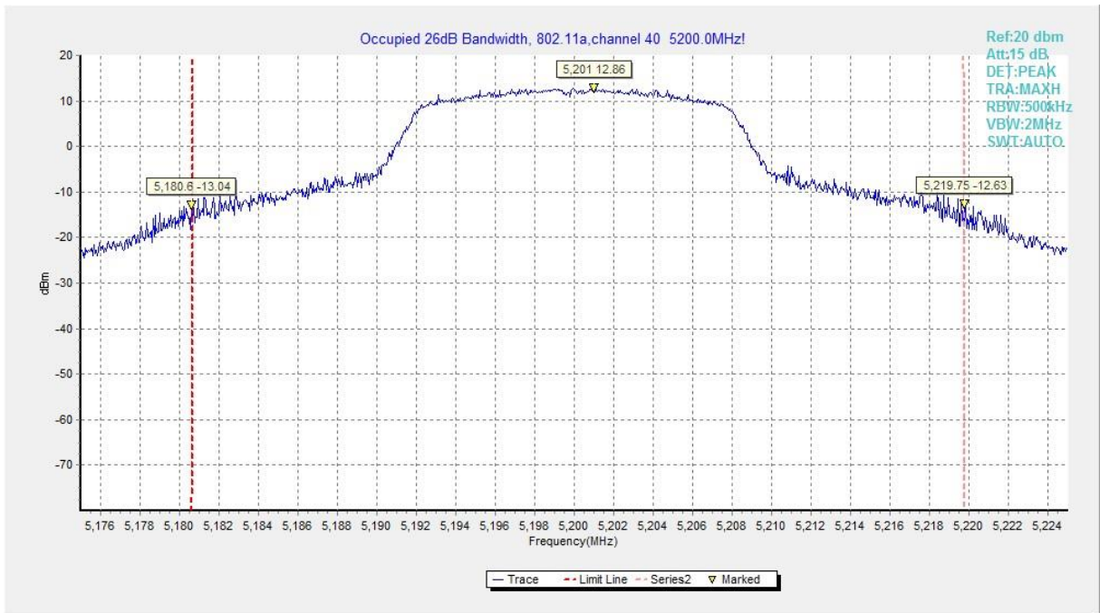
Fig.2 Occupied 26dB Bandwidth (802.11a, 5200MHz)
