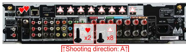
(2) Remove the connector PCB.
