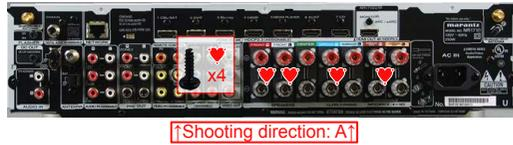
(2) Remove the screws. Remove the CORD HOLDER and connectors. Remove the HOLDER.
