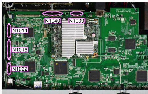
(3) Remove the DIGITAL PCB from the chassis and turn it over.
