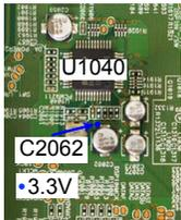
**Check item(3-9.2).** Check the power supply voltage.:
