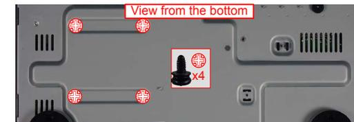
NOTE : It will separate and TRANS will fall from SET, if screws is removed.
