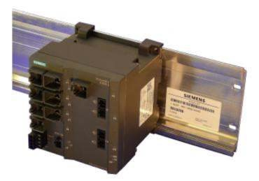
Installing an IE Switch X-300 on a SIMATIC S7-300 standard rail Figure 5-2
