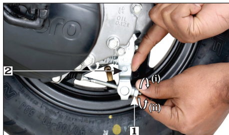
(1) Adjuster nut (2) Brake arm (i) Decrease free play (ii) Increase free play
