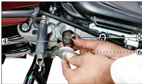
(4) Spring (5) Oil strainer screen (6) O-ring
