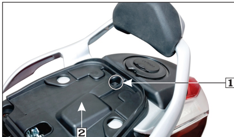
(1) Bolt (2) Fuel tray sub assembly
