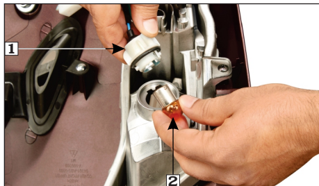
(1) Bulb holder (2) Front turn signal bulb
