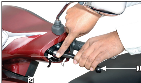
(1) Integrated brake lever (2) Lever lock
