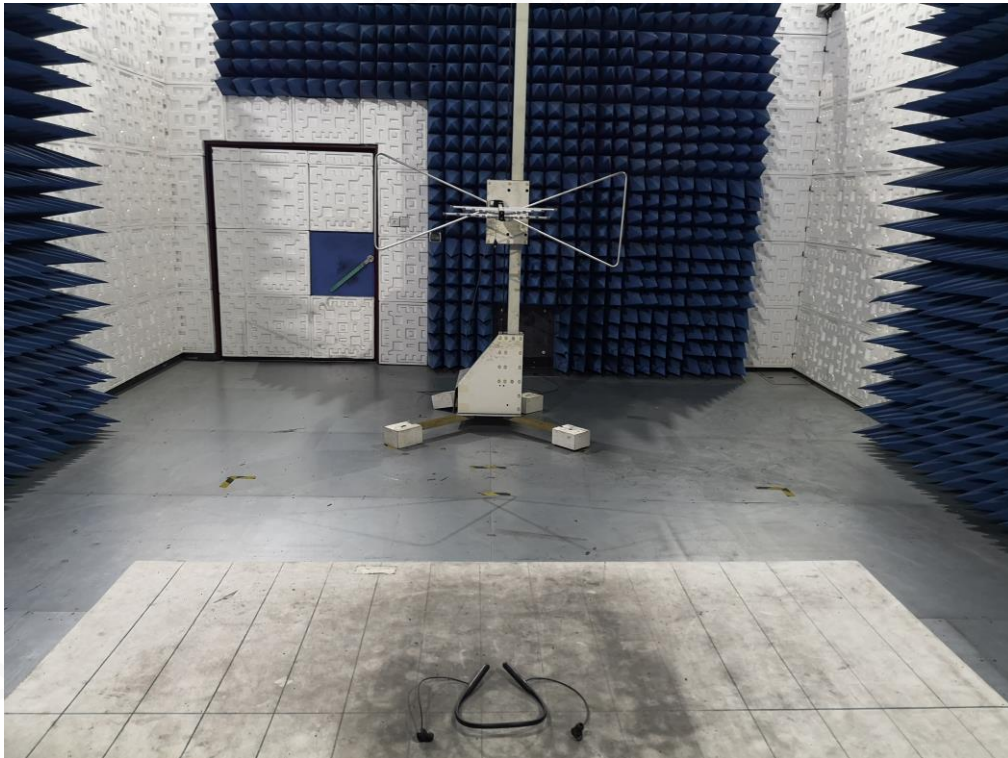
RADIATED EMISSION TEST SETUP ABOVE 1GHZ
