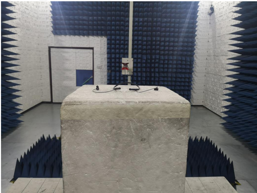
RADIATED EMISSION TEST SETUP ABOVE 1GHZ
