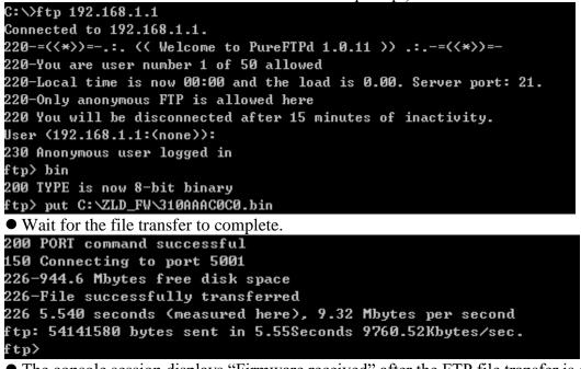
• The console session displays "Firmware received" after the FTP file transfer is complete. Then you need to wait while the ZyWALL/USG recovers the firmware (this may take up to 4 minutes).
