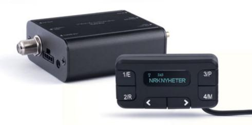
The Tiny Audio C11+ has a separate receiver unit that can be concealed.
