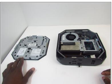
While holding the latch, lift the access panel upwards and towards yourself and set it aside upsidedown.
