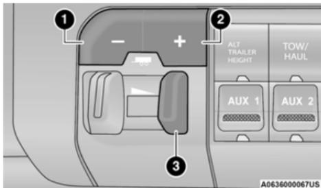
**Integrated Trailer Brake Module (ITBM)**
