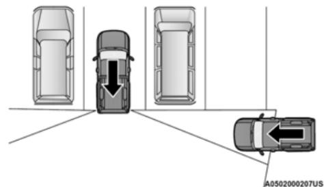
RCP monitors the rear detection zones on both sides of the vehicle, for objects that are moving toward the side of the vehicle with a minimum speed of approximately 3 mph (5 km/h), to objects moving a maximum of approximately 20 mph (32 km/h), such as in parking lot situations.
