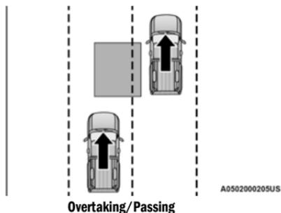
The BSM system is designed not to issue an alert on stationary objects such as guardrails, posts, walls, foliage, berms, snow banks, car washes, etc. However, occasionally the system may alert on such objects. This is normal operation and your vehicle does not require service.
