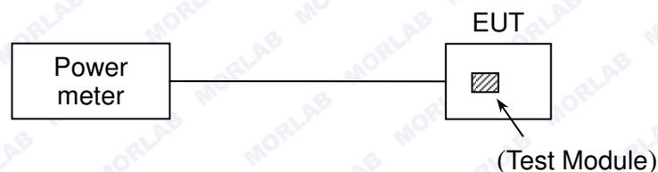
The EUT (Equipment under the test) which is coupled to the Power Meter; the RF load attached to the EUT antenna terminal is 50Ohm; the path loss as the factor is calibrated to correct the reading, all test result in power meter.
