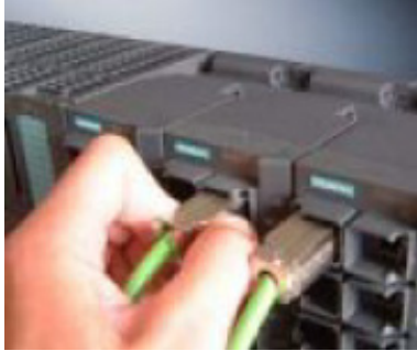
Figure 5-4 Releasing the RJ-45 Plug
