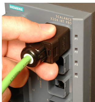
Figure 5-8 Removing IE RJ 45 Plug Pro or IE SC RJ Plug Pro
