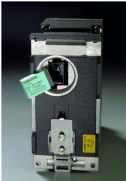
Figure 3-44 Removing the C-PLUG from the receptacle
