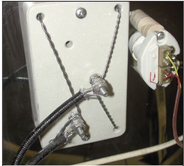
Photo of element terminal with elements and Power Lead Wires shown connected.
