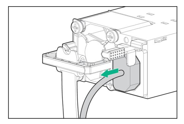
b. Remove the power supply.
