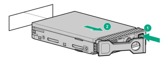
Removing and replacing media devices
