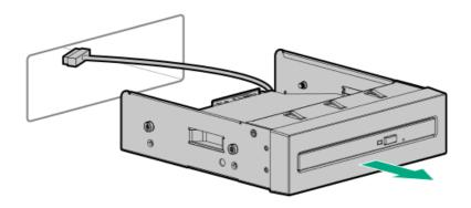
10. Remove the optical drive from the optical drive cage.
