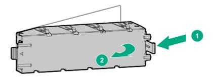
To replace the component, insert the tab on the blank into the slot on the media bay.
