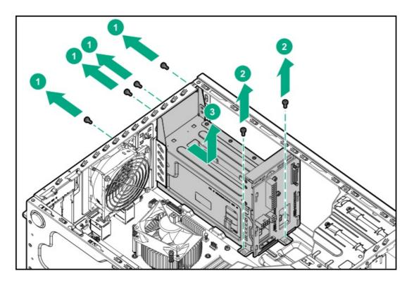
11. Remove the Flexible Slot power supply backplane.
