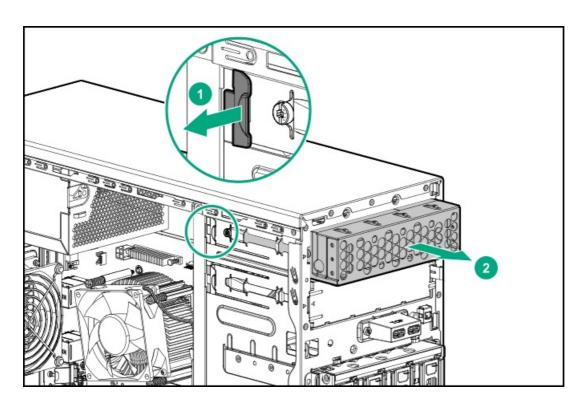
11. Remove the screws and slide out the drive from the drive enablement assembly.
