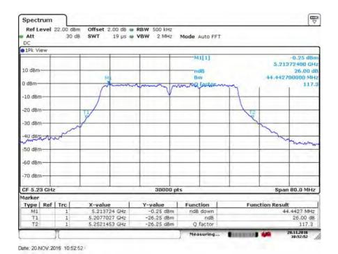
Test mode: 802.11ac(HT40) MIMO Frequency(MHz): 5270
