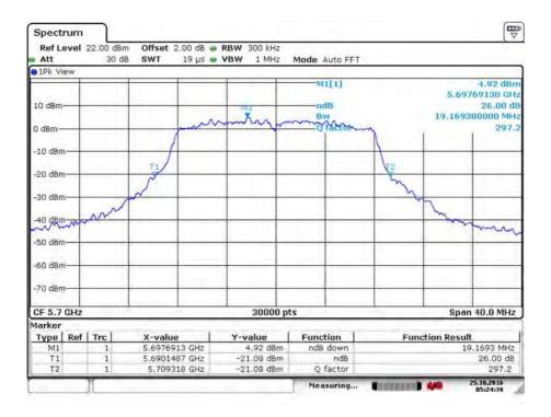
Test mode: 802.11n(HT20) Frequency(MHz): 5180
