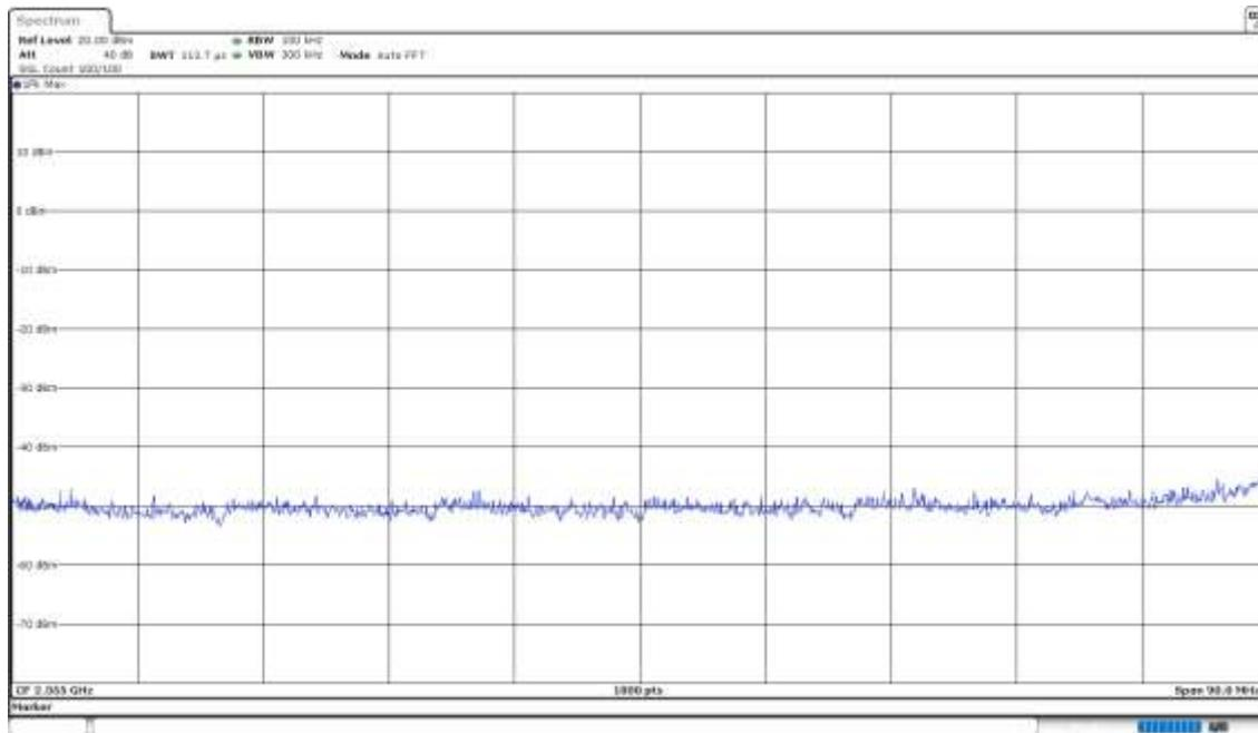
**Operation Band (MHz) = [2400, 2483.5], Frequency (MHz) = 2462.00, Equipment Type: Digital Transmission System (DTS), Modulation: 802.11n HT20 (OFDM MCS0 6.5 Mbit/s)**
