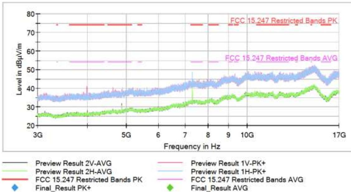
**Operation Band (MHz) = [2400, 2483.5], Frequency (MHz) = 2462.00000, Equipment Type: Digital Transmission System (DTS), Modulation: 802.11b (DSSS 1 Mbit/s), Frequency Range (GHz) = [3, 17]**
