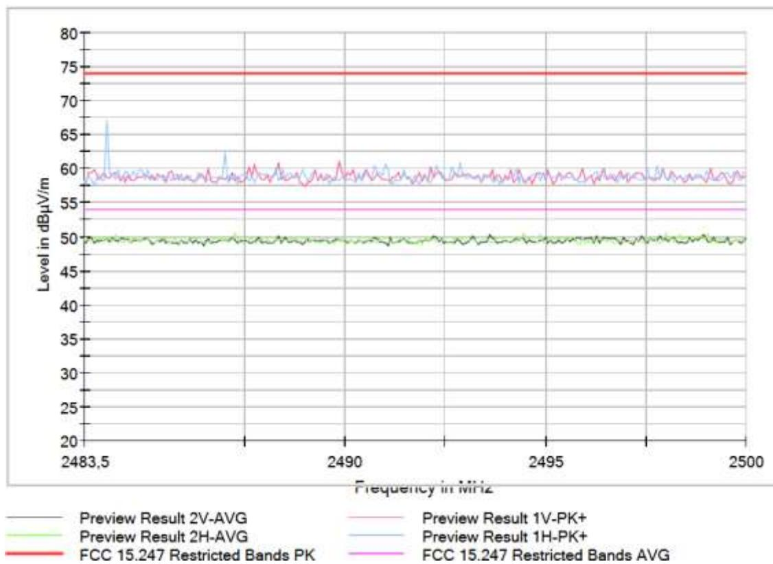
**Operation Band (MHz) = [2400, 2483.5], Frequency (MHz) = 2412.00000, Equipment Type: Digital Transmission System (DTS), Modulation: 802.11n HT20 (OFDM MCS0 6.5 Mbit/s), Frequency Range (GHz) = [3, 17]**
