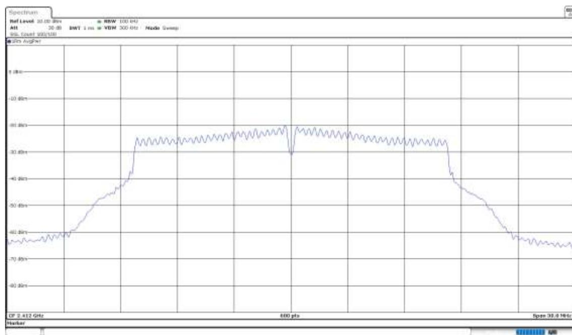
**Operation Band (MHz) = [2400, 2483.5], Frequency (MHz) = 2437.00000, Equipment Type: Digital Transmission System (DTS), Modulation: 802.11g (OFDM 6 Mbit/s)**
