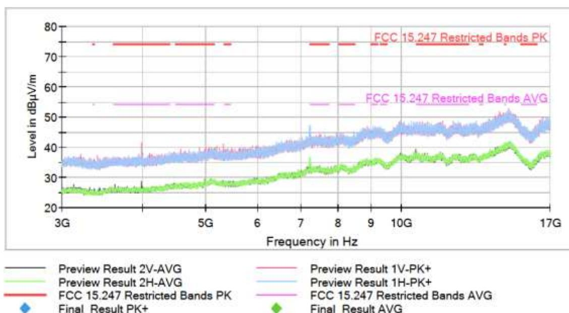
**Operation Band (MHz) = [2400, 2483.5], Frequency (MHz) = 2437.00000, Equipment Type: Digital Transmission System (DTS), Modulation: 802.11g (OFDM 6 Mbit/s), Frequency Range (GHz) = [3, 17]**
