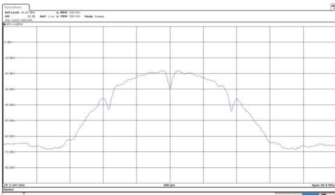
**Operation Band (MHz) = [2400, 2483.5], Frequency (MHz) = 2462.00000, Equipment Type: Digital Transmission System (DTS), Modulation: 802.11b (DSSS 1 Mbit/s)**
