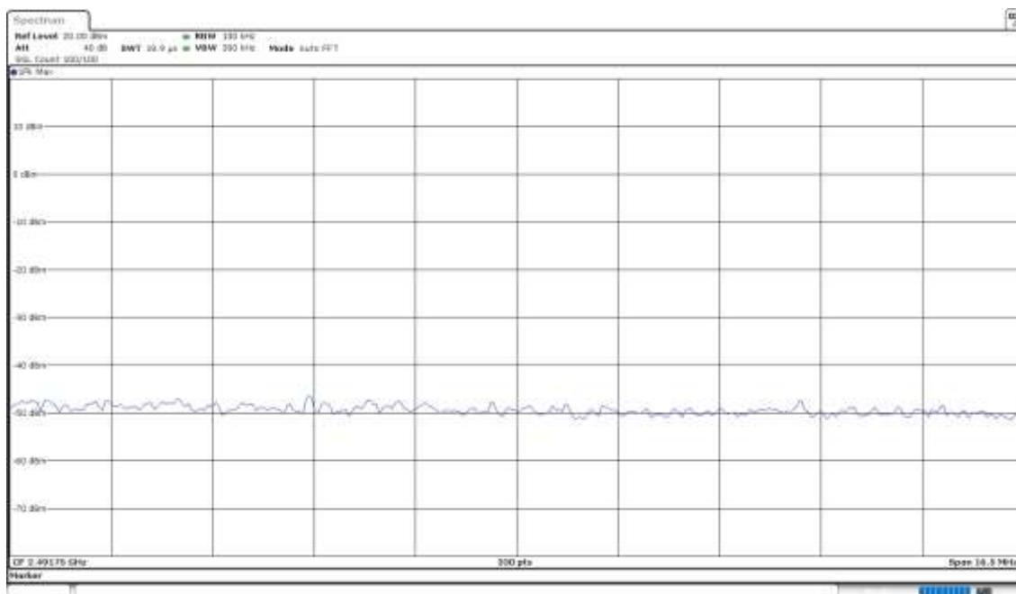
**Operation Band (MHz) = [2400, 2483.5], Frequency (MHz) = 2412.00, Equipment Type: Digital Transmission System (DTS), Modulation: 802.11n HT20 (OFDM MCS0 6.5 Mbit/s)**
