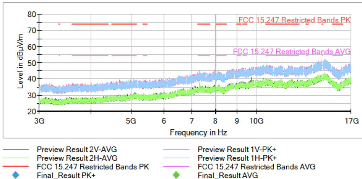
Operation Band (MHz) = [2400, 2483.5], Frequency (MHz) = 2462.00000, Equipment Type: Digital Transmission System (DTS), Modulation: 802.11g (OFDM 6 Mbit/s), Frequency Range (GHz) = [3, 17]
