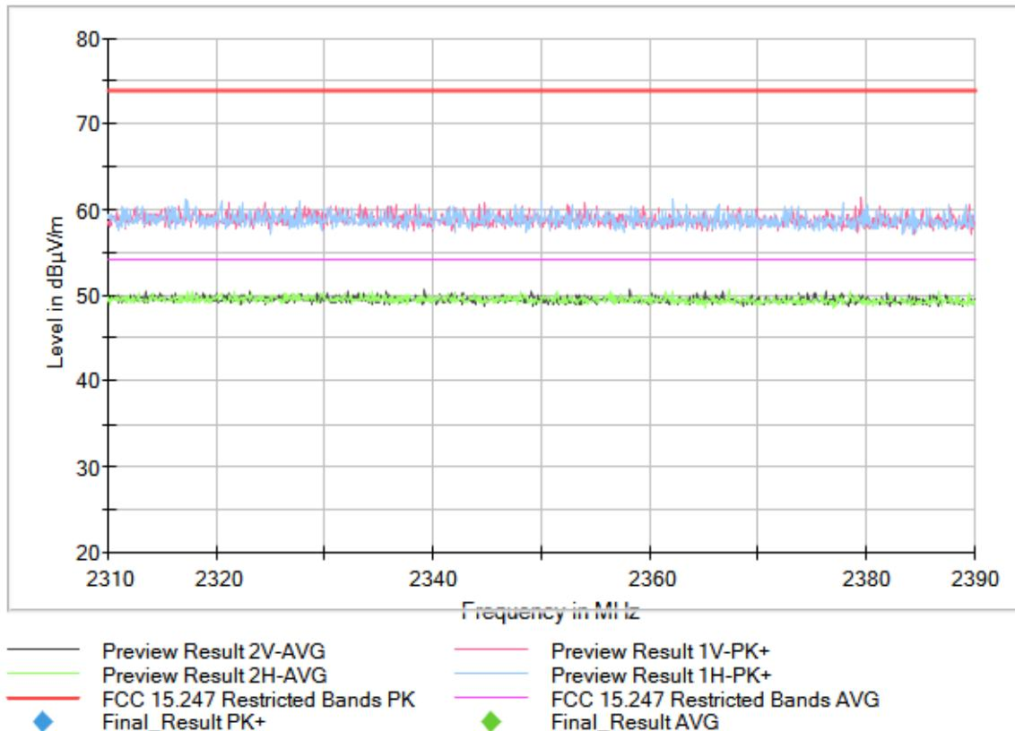
**Operation Band (MHz) = [2400, 2483.5], Frequency (MHz) = 2437.00000, Equipment Type: Digital Transmission System (DTS), Modulation: 802.11b (DSSS 1 Mbit/s), Frequency Range (GHz) = [1, 3]**
