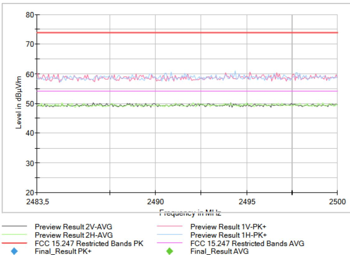
Operation Band (MHz) = [2400, 2483.5], Frequency (MHz) = 2462.00000, Equipment Type: Digital Transmission System (DTS), Modulation: 802.11n HT20 (OFDM MCS0 6.5 Mbit/s), Frequency Range (GHz) = [1, 3]
