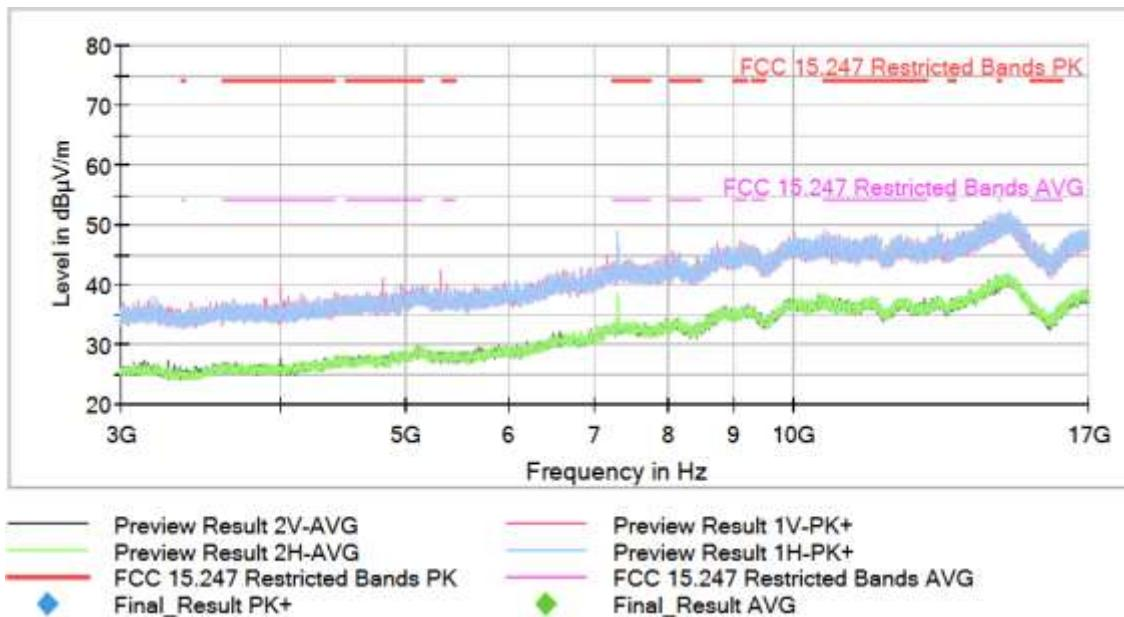
**Operation Band (MHz) = [2400, 2483.5], Frequency (MHz) = 2462.00000, Equipment Type: Digital Transmission System (DTS), Modulation: 802.11g (OFDM 6 Mbit/s), Frequency Range (GHz) = [3, 17]**
