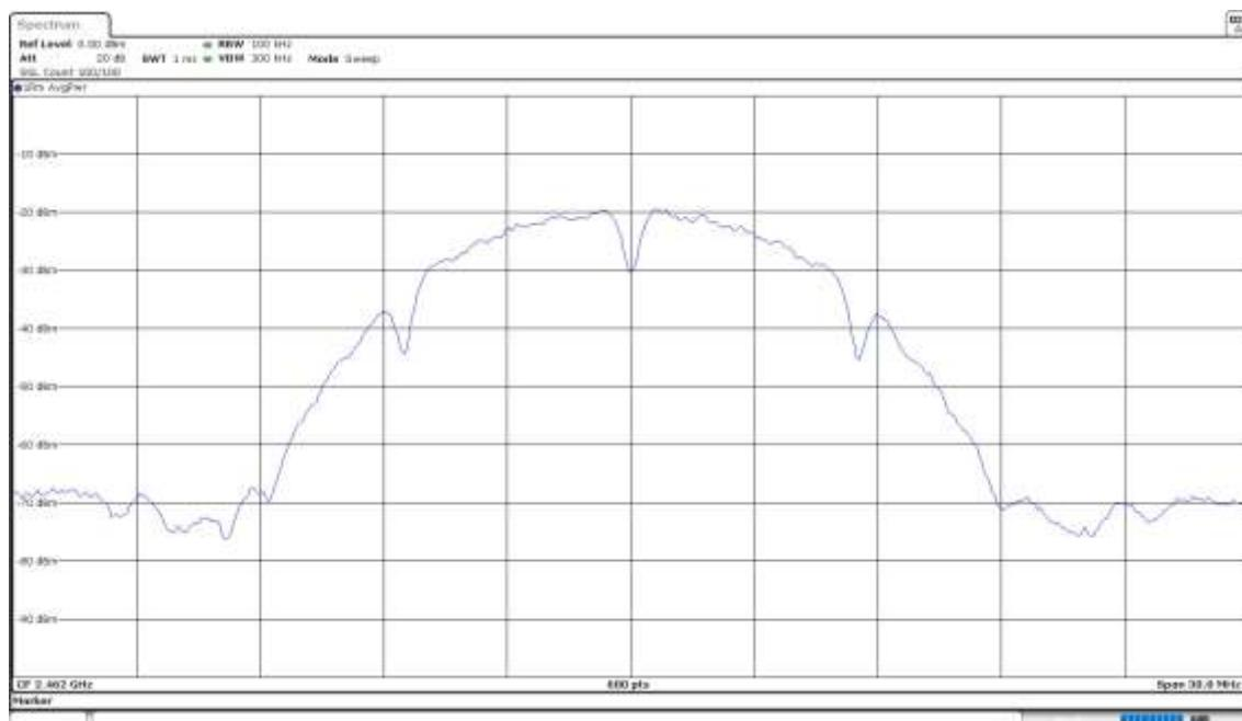
**Operation Band (MHz) = [2400, 2483.5], Frequency (MHz) = 2412.00000, Equipment Type: Digital Transmission System (DTS), Modulation: 802.11g (OFDM 6 Mbit/s)**
