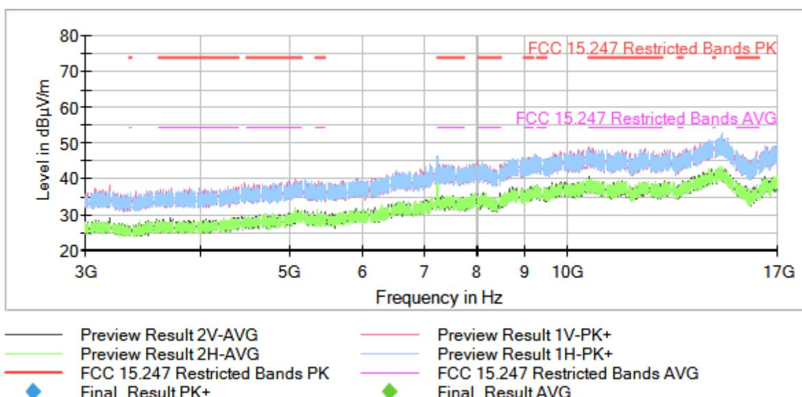
Operation Band (MHz) = [2400, 2483.5], Frequency (MHz) = 2437.00000, Equipment Type: Digital Transmission System (DTS), Modulation: 802.11n HT20 (OFDM MCS0 6.5 Mbit/s), Frequency Range (GHz) = [3, 17]
