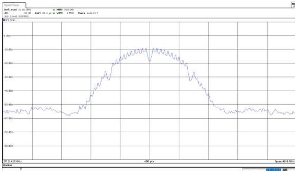
**Operation Band (MHz) = [2400, 2483.5], Frequency (MHz) = 2437.00000, Equipment Type: Digital Transmission System (DTS), Modulation: 802.11b (DSSS 1 Mbit/s)**
