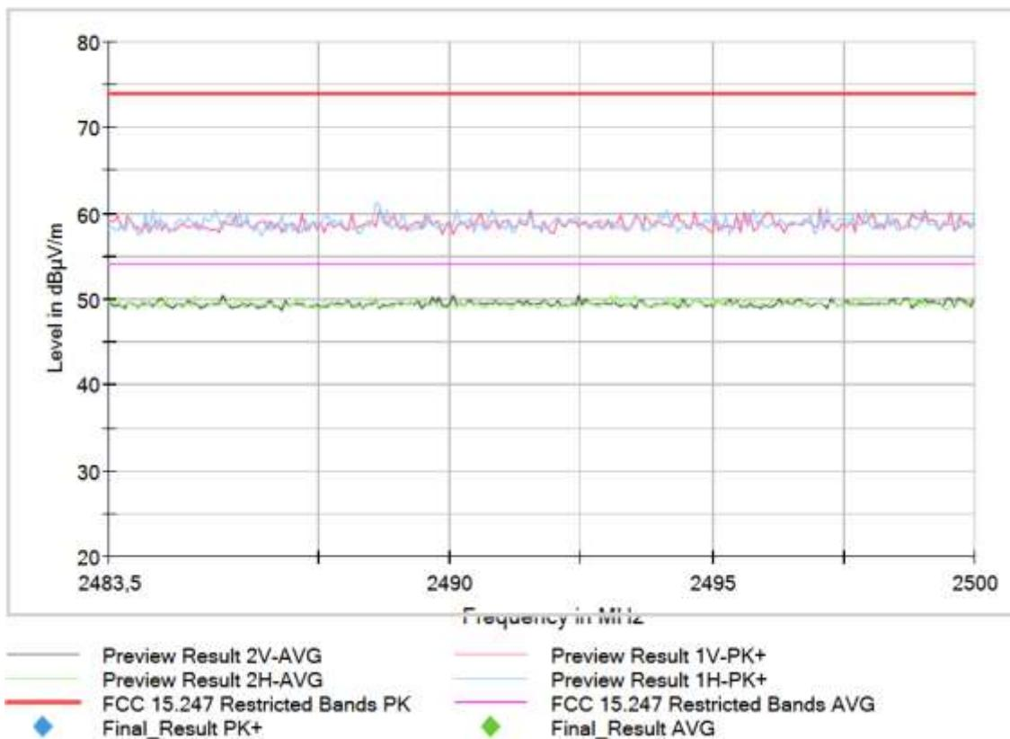
**Operation Band (MHz) = [2400, 2483.5], Frequency (MHz) = 2462.00000, Equipment Type: Digital Transmission System (DTS), Modulation: 802.11g (OFDM 6 Mbit/s), Frequency Range (GHz) = [1, 3]**
