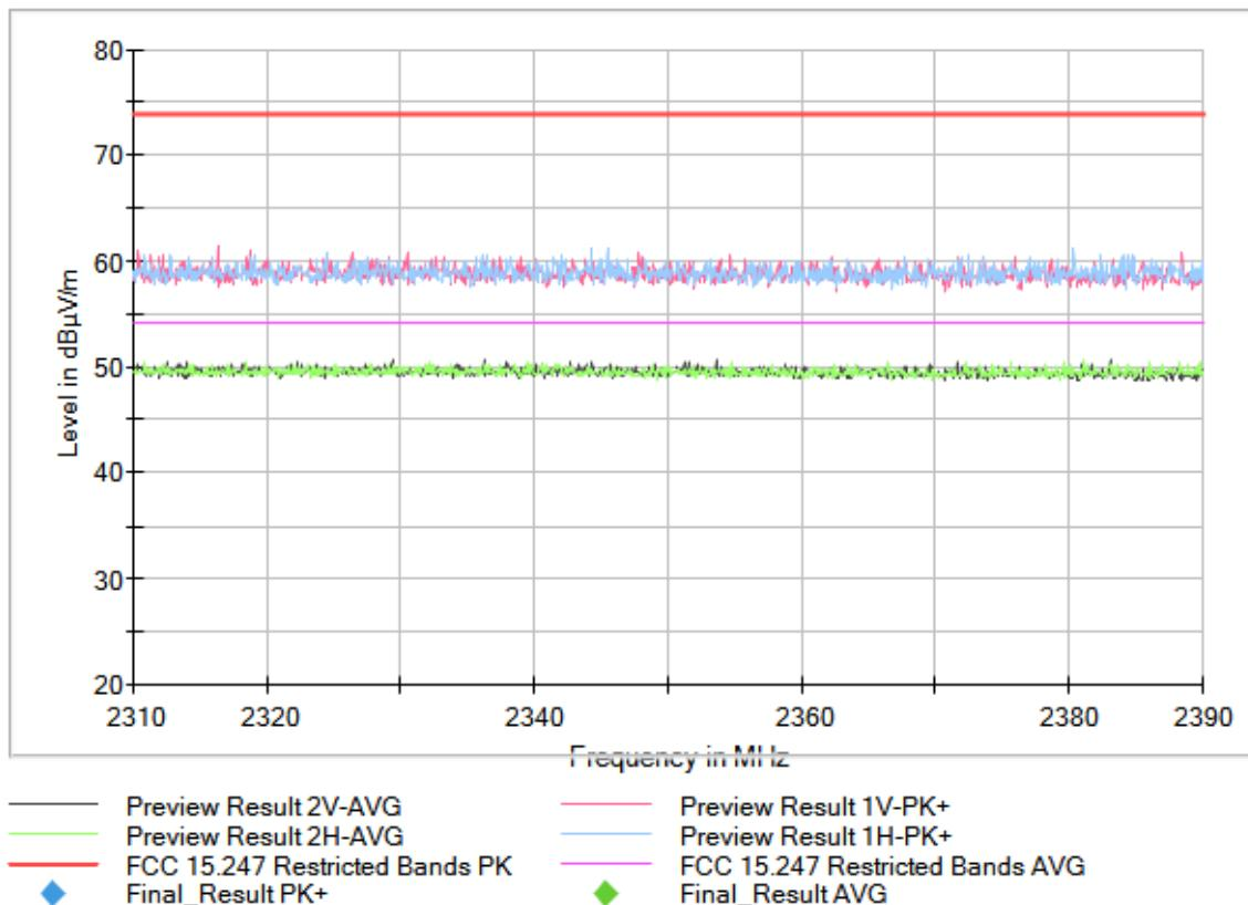
**Operation Band (MHz) = [2400, 2483.5], Frequency (MHz) = 2437.00000, Equipment Type: Digital Transmission System (DTS), Modulation: 802.11g (OFDM 6 Mbit/s), Frequency Range (GHz) = [1, 3]**
