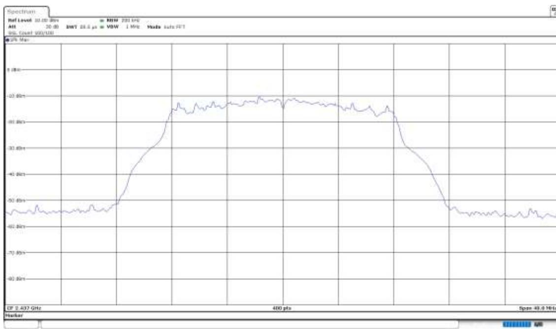
**Operation Band (MHz) = [2400, 2483.5], Frequency (MHz) = 2462.00000, Equipment Type: Digital Transmission System (DTS), Modulation: 802.11g (OFDM 6 Mbit/s)**
