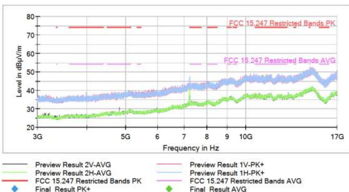
**Operation Band (MHz) = [2400, 2483.5], Frequency (MHz) = 2437.00000, Equipment Type: Digital Transmission System (DTS), Modulation: 802.11b (DSSS 1 Mbit/s), Frequency Range (GHz) = [3, 17]**
