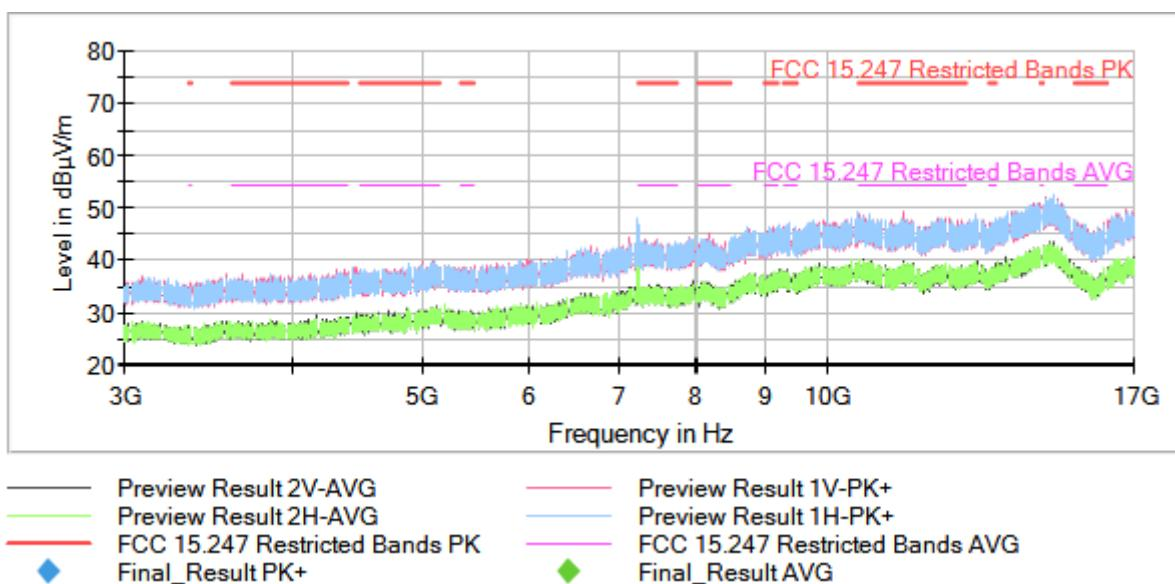
Operation Band (MHz) = [2400, 2483.5], Frequency (MHz) = 2437.00000, Equipment Type: Digital Transmission System (DTS), Modulation: 802.11g (OFDM 6 Mbit/s), Frequency Range (GHz) = [3, 17]
