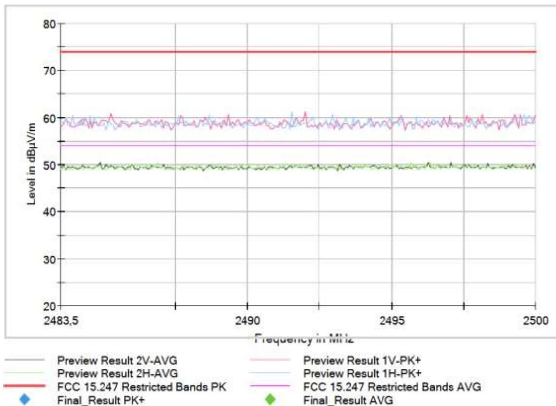
**Operation Band (MHz) = [2400, 2483.5], Frequency (MHz) = 2437.00000, Equipment Type: Digital Transmission System (DTS), Modulation: 802.11n HT20 (OFDM MCS0 6.5 Mbit/s), Frequency Range (GHz) = [1, 3]**
