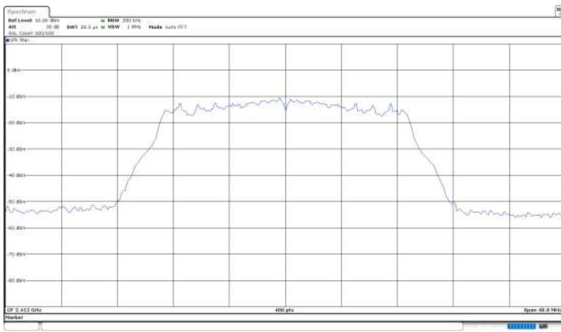
**Operation Band (MHz) = [2400, 2483.5], Frequency (MHz) = 2437.00000, Equipment Type: Digital Transmission System (DTS), Modulation: 802.11n HT20 (OFDM MCS0 6.5 Mbit/s)**
