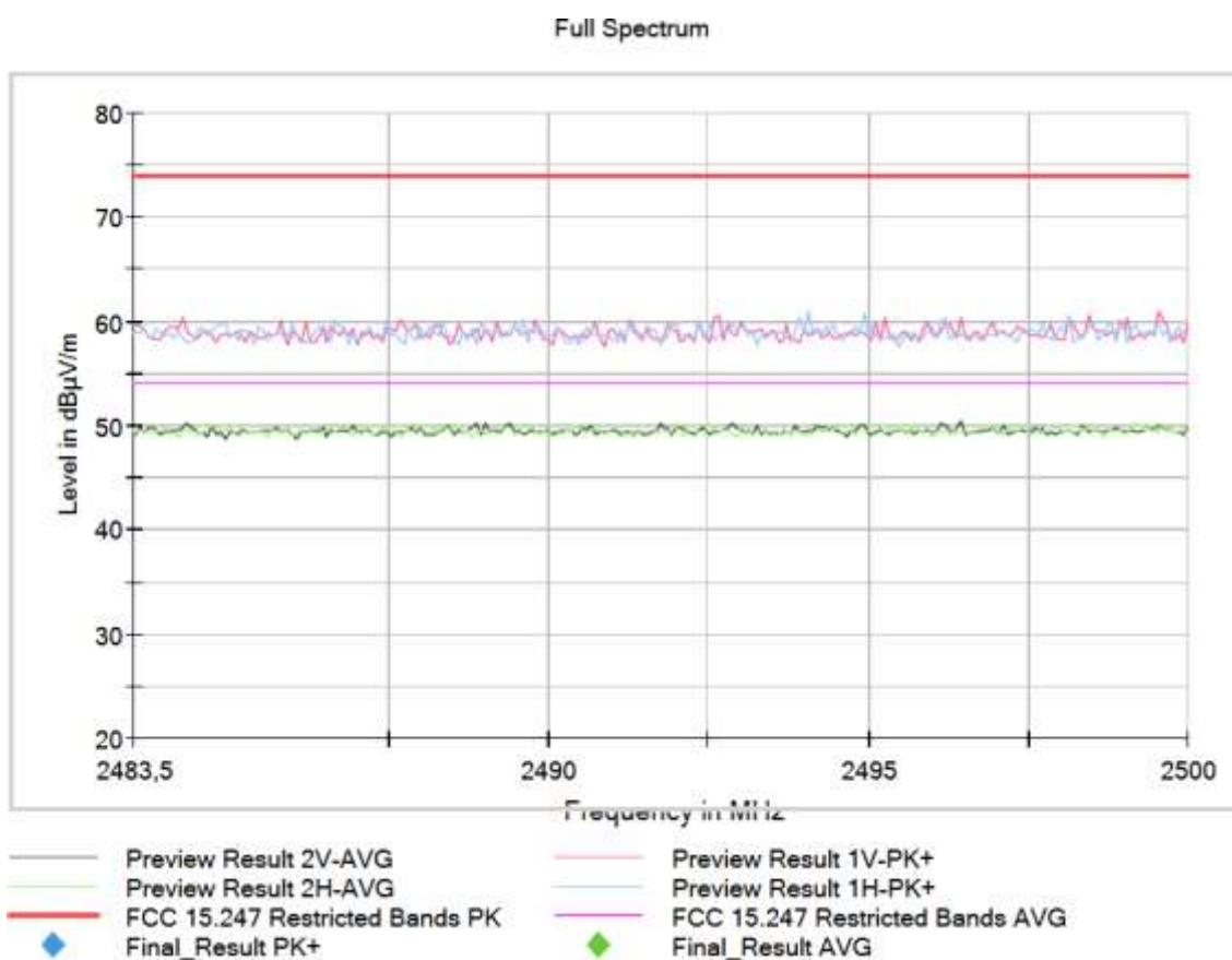
**Operation Band (MHz) = [2400, 2483.5], Frequency (MHz) = 2437.00000, Equipment Type: Digital Transmission System (DTS), Modulation: 802.11b (DSSS 1 Mbit/s), Frequency Range (GHz) = [1, 3]**
