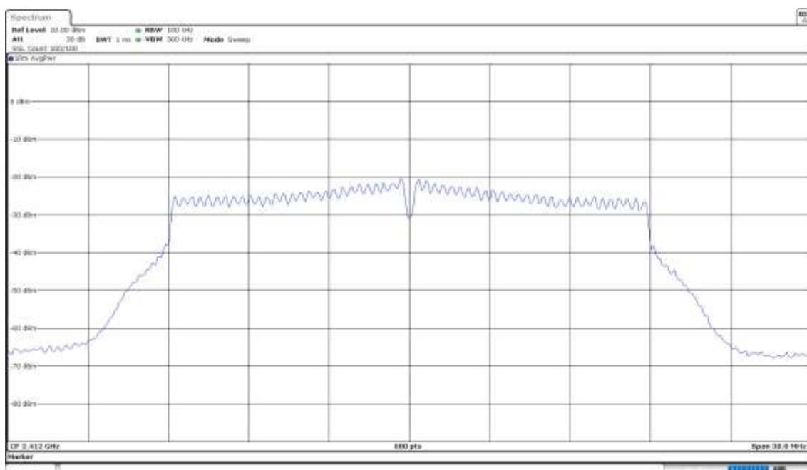
**Operation Band (MHz) = [2400, 2483.5], Frequency (MHz) = 2437.00000, Equipment Type: Digital Transmission System (DTS), Modulation: 802.11n HT20 (OFDM MCS0 6.5 Mbit/s)**
