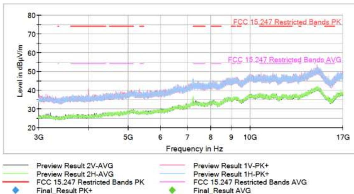
Operation Band (MHz) = [2400, 2483.5], Frequency (MHz) = 2437.00000, Equipment Type: Digital Transmission System (DTS), Modulation: 802.11n HT20 (OFDM MCS0 6.5 Mbit/s), Frequency Range (GHz) = [3, 17]
