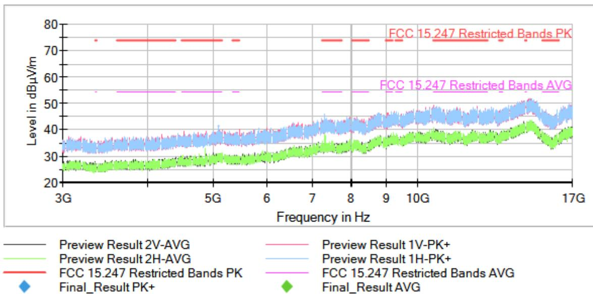
Operation Band (MHz) = [2400, 2483.5], Frequency (MHz) = 2462.00000, Equipment Type: Digital Transmission System (DTS), Modulation: 802.11b (DSSS 1 Mbit/s), Frequency Range (GHz) = [3, 17]
