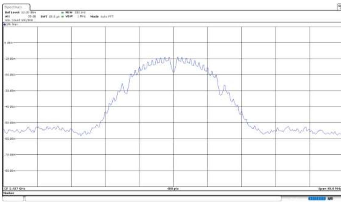
**Operation Band (MHz) = [2400, 2483.5], Frequency (MHz) = 2462.00000, Equipment Type: Digital Transmission System (DTS), Modulation: 802.11b (DSSS 1 Mbit/s)**
