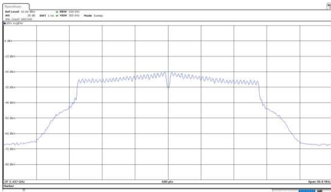
**Operation Band (MHz) = [2400, 2483.5], Frequency (MHz) = 2462.00000, Equipment Type: Digital Transmission System (DTS), Modulation: 802.11g (OFDM 6 Mbit/s)**
