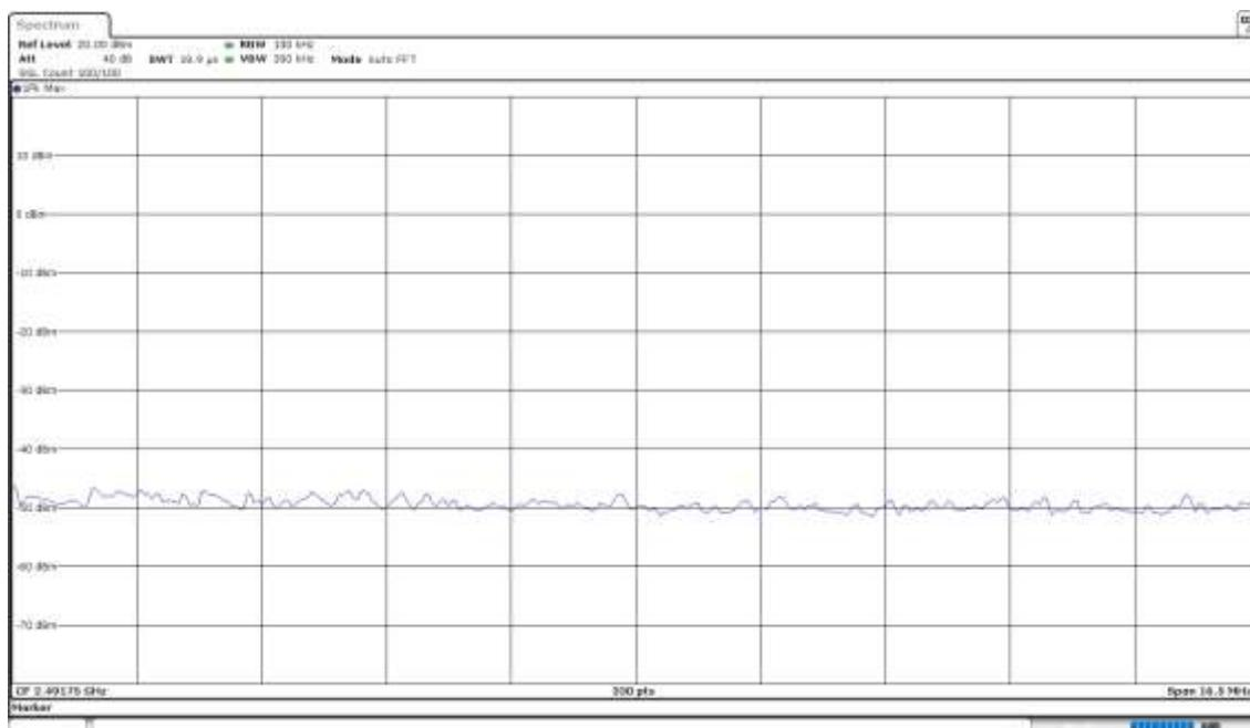
**Operation Band (MHz) = [2400, 2483.5], Frequency (MHz) = 2412.00, Equipment Type: Digital Transmission System (DTS), Modulation: 802.11g (OFDM 6 Mbit/s)**
