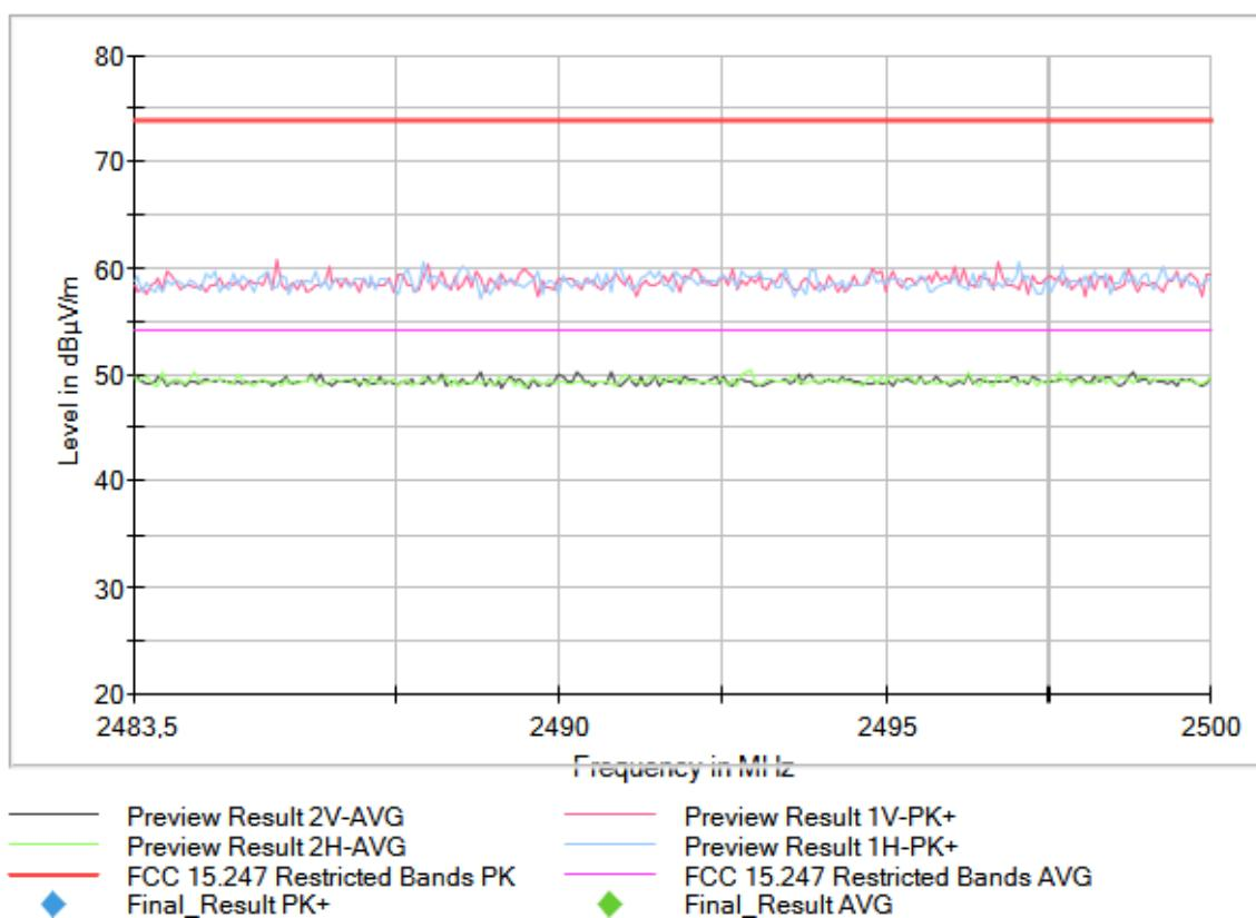
**Operation Band (MHz) = [2400, 2483.5], Frequency (MHz) = 2462.00000, Equipment Type: Digital Transmission System (DTS), Modulation: 802.11b (DSSS 1 Mbit/s), Frequency Range (GHz) = [1, 3]**
