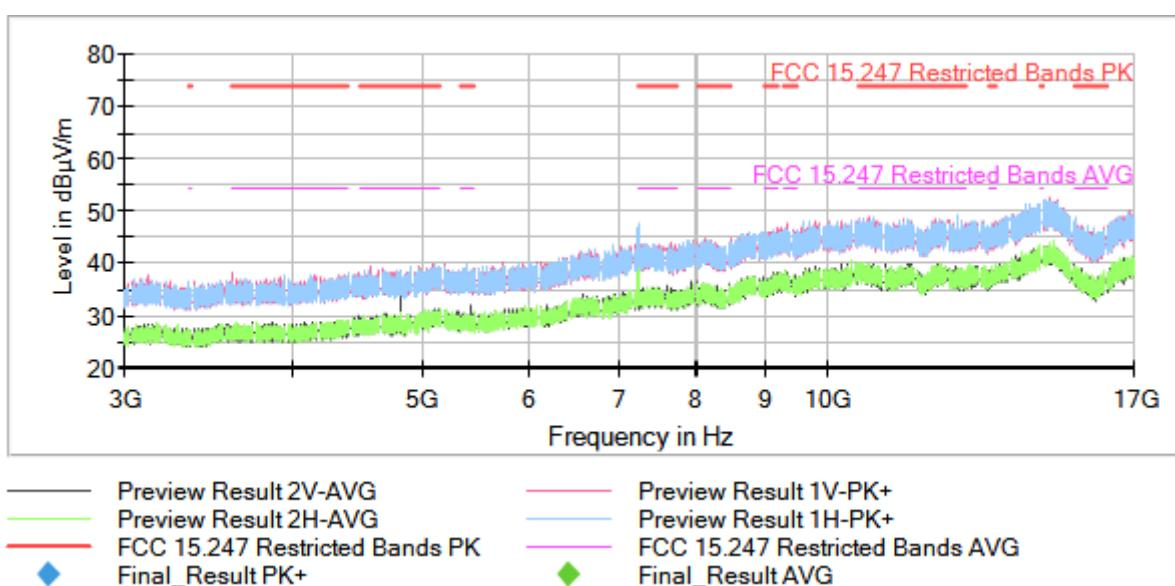
Operation Band (MHz) = [2400, 2483.5], Frequency (MHz) = 2437.00000, Equipment Type: Digital Transmission System (DTS), Modulation: 802.11b (DSSS 1 Mbit/s), Frequency Range (GHz) = [3, 17]
