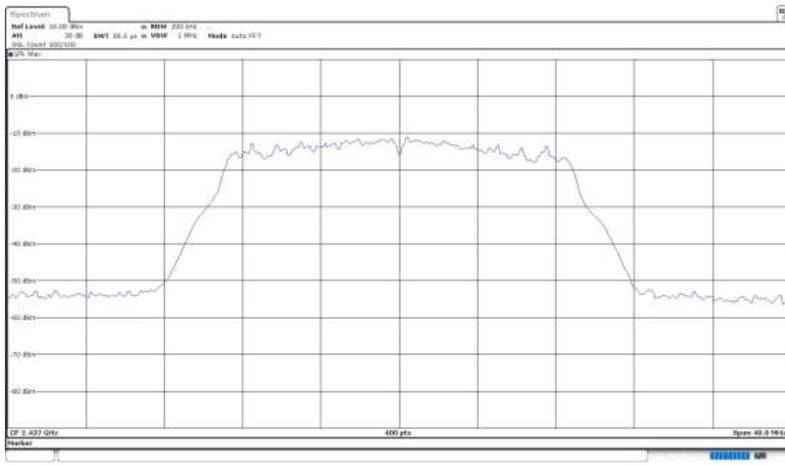
**Operation Band (MHz) = [2400, 2483.5], Frequency (MHz) = 2462.00000, Equipment Type: Digital Transmission System (DTS), Modulation: 802.11n HT20 (OFDM MCS0 6.5 Mbit/s)**
