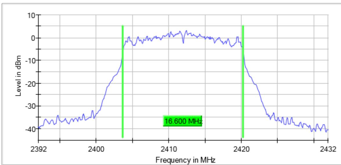
**Operation Band (MHz) = [2400, 2483.5], Frequency (MHz) = 2437.00000, Equipment Type: Digital Transmission System (DTS), Modulation: 802.11g (OFDM 6 Mbit/s)**
