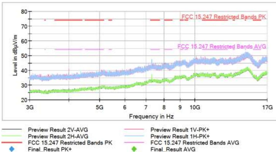
Operation Band (MHz) = [2400, 2483.5], Frequency (MHz) = 2462.00000, Equipment Type: Digital Transmission System (DTS), Modulation: 802.11n HT20 (OFDM MCS0 6.5 Mbit/s), Frequency Range (GHz) = [3, 17]
