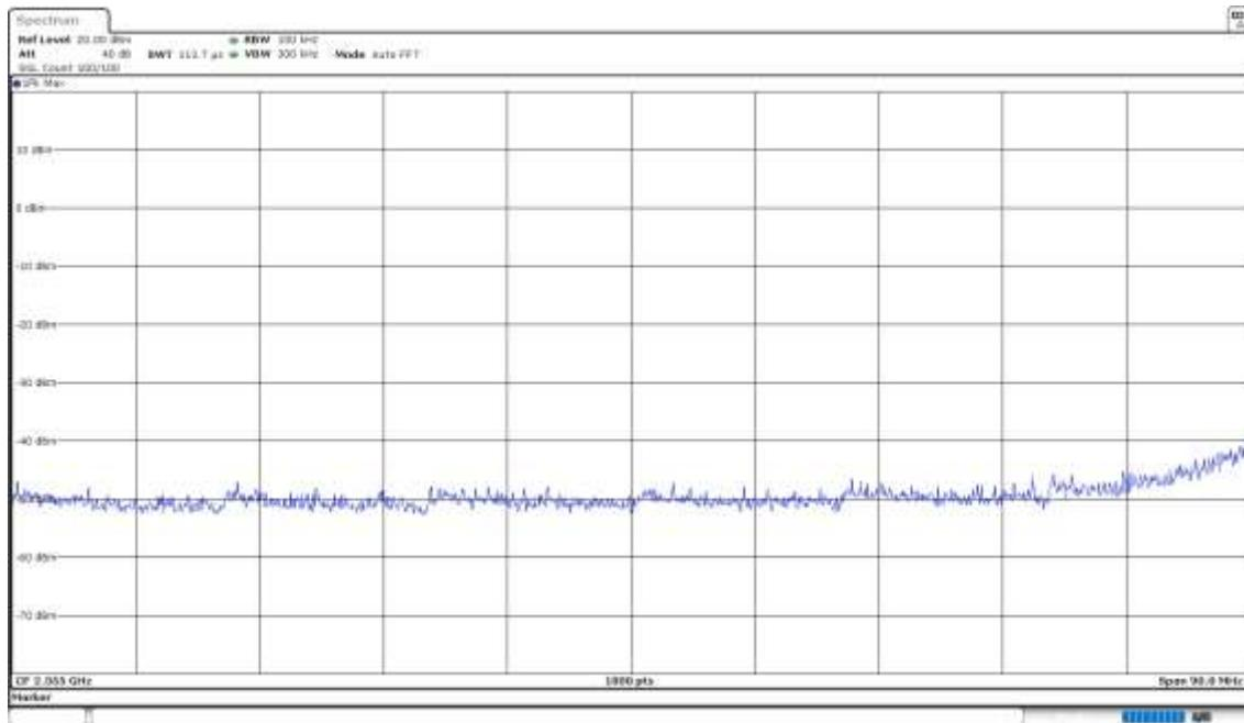
**Operation Band (MHz) = [2400, 2483.5], Frequency (MHz) = 2462.00, Equipment Type: Digital Transmission System (DTS), Modulation: 802.11g (OFDM 6 Mbit/s)**
