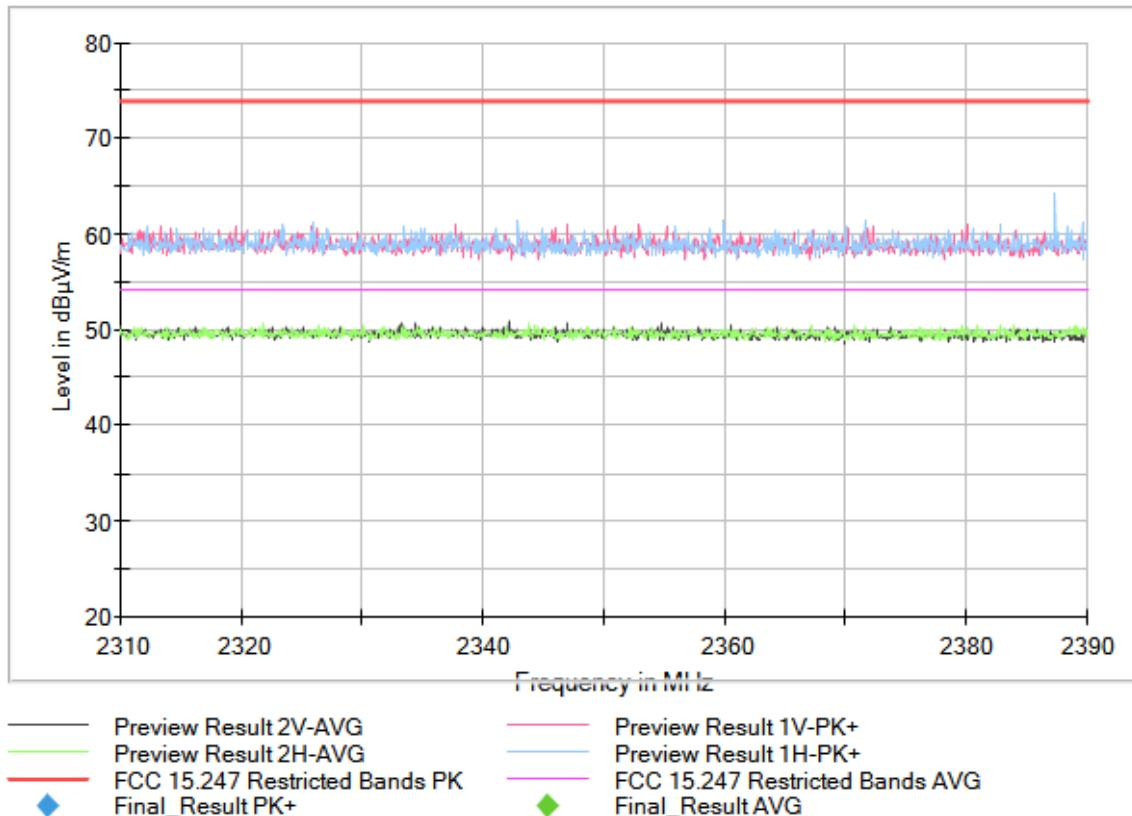
**Operation Band (MHz) = [2400, 2483.5], Frequency (MHz) = 2437.00000, Equipment Type: Digital Transmission System (DTS), Modulation: 802.11n HT20 (OFDM MCS0 6.5 Mbit/s), Frequency Range (GHz) = [1, 3]**
