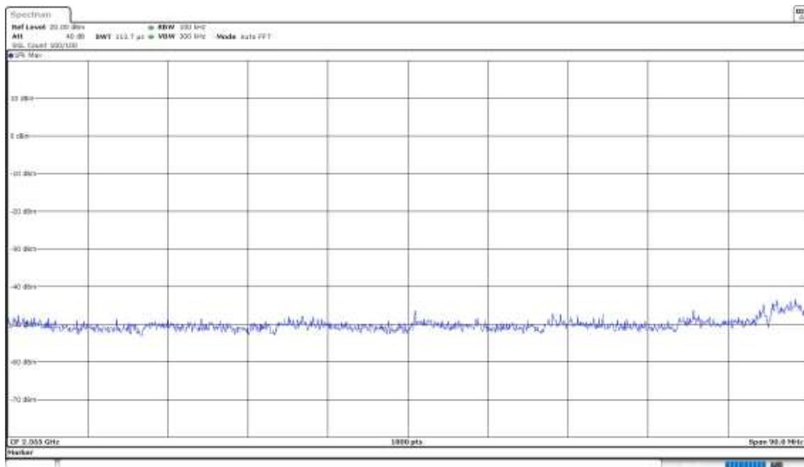
**Operation Band (MHz) = [2400, 2483.5], Frequency (MHz) = 2462.00, Equipment Type: Digital Transmission System (DTS), Modulation: 802.11b (DSSS 1 Mbit/s)**
