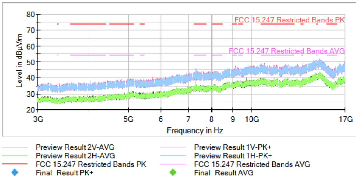
Operation Band (MHz) = [2400, 2483.5], Frequency (MHz) = 2462.00000, Equipment Type: Digital Transmission System (DTS), Modulation: 802.11n HT20 (OFDM MCS0 6.5 Mbit/s), Frequency Range (GHz) = [3, 17]
