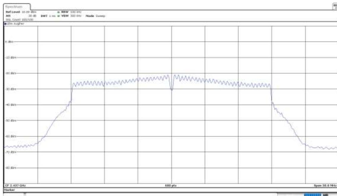
**Operation Band (MHz) = [2400, 2483.5], Frequency (MHz) = 2462.00000, Equipment Type: Digital Transmission System (DTS), Modulation: 802.11n HT20 (OFDM MCS0 6.5 Mbit/s)**
