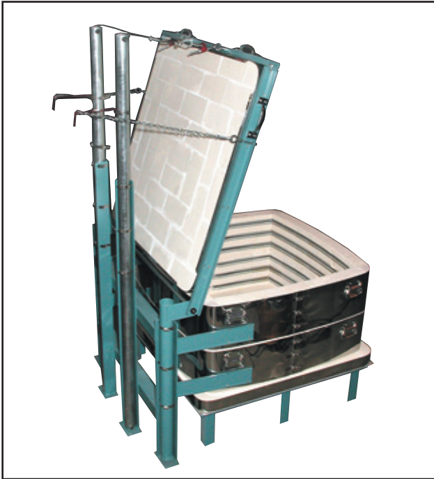
A DaVinci with lid up and safety chains on
