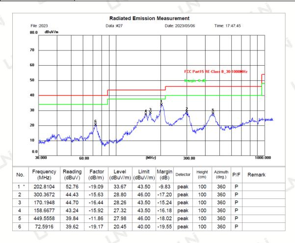
Remark: Absolute Level = Reading Level + Factor, Margin = Absolute Level - Limit Factor = Ant. Factor + Cable Loss - Pre-amplifier
