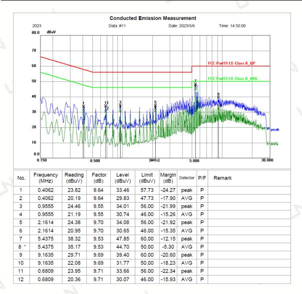
Remark:1. Factor = Insertion Loss + Cable Loss, Result = Reading + Factor, Margin = Result – Limit.
