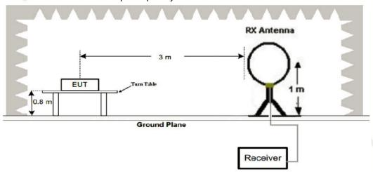
2. Radiated Emission Test-Up Frequency 30MHz~1GHz
