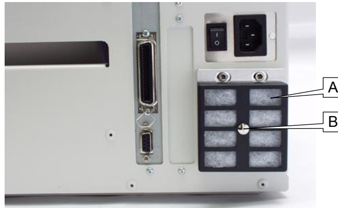
Fig. 7 64-08 with mounted dust filter (A).
