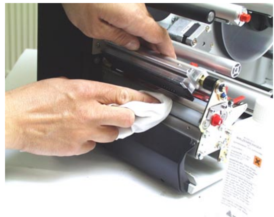
Fig. 4 Rotate the printhead upwards before cleaning it.
