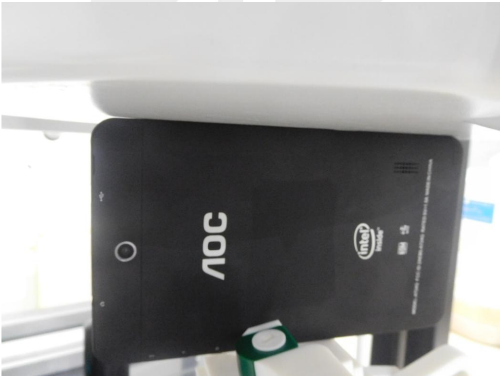
Body left side(separation distance is 0mm)
