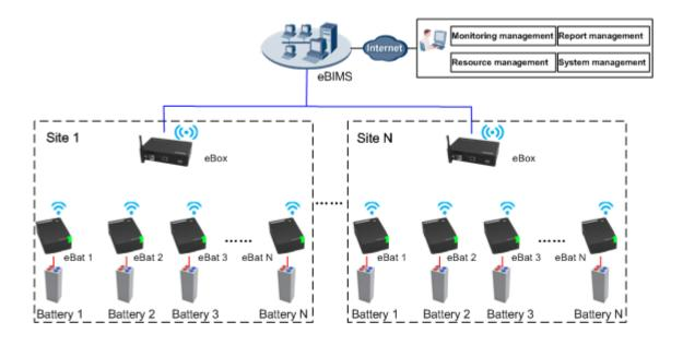
The eBIMS uses modular deployment. The typical configuration includes the software system, a set of matched hardware, multiple eBats, and one eBox. The number of eBats is determined by the eBox management capacity and the battery quantity. One eBat is used for each battery. There are 2 V and 12 V batteries
