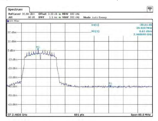
802.11n-HT40 Channel 03 (2422MHz) Reference Level: -3.48dBm
