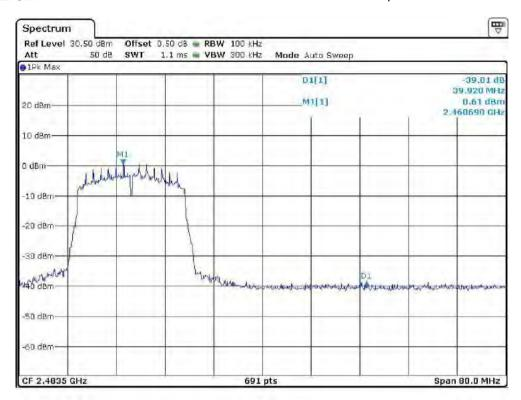
802.11n-HT40 Channel 03 (2422MHz) Reference Level: -3.26dBm
