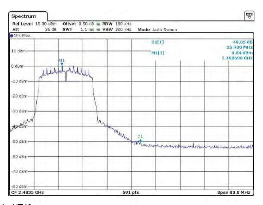
802.11n-HT40 Channel 03 (2422MHz) Reference Level: -3.53dBm
