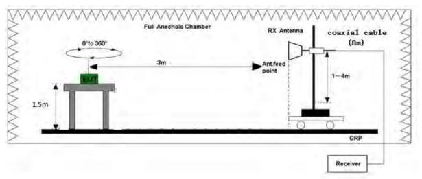
Test set-up of radiated disturbance (Above 1GHz)
