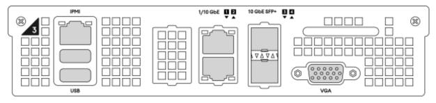
The IPMI, USB, and VGA ports are only needed for advanced diagnostics. IPMI allows accessing the nodes over the network for out-of-band management via a remote console. The default IPMI password to access the management node via SSH is **Acronis!Infra%30** (it changes to a user-specified password during deployment). The USB and VGA ports allow you to connect a keyboard and a monitor to a node if the network is unavailable.
